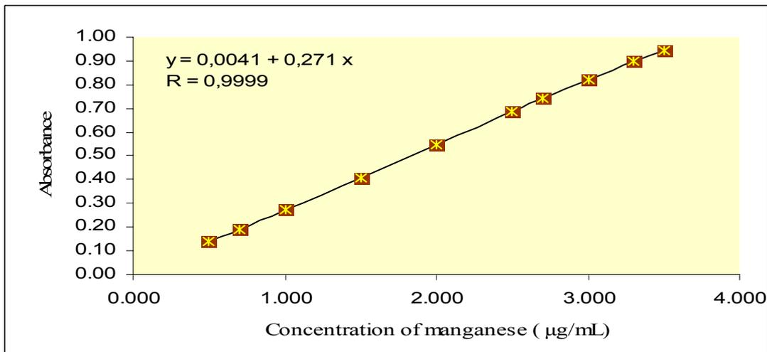
Fig. 2 – The calibration curve for Mn determination through f\_AAS.
