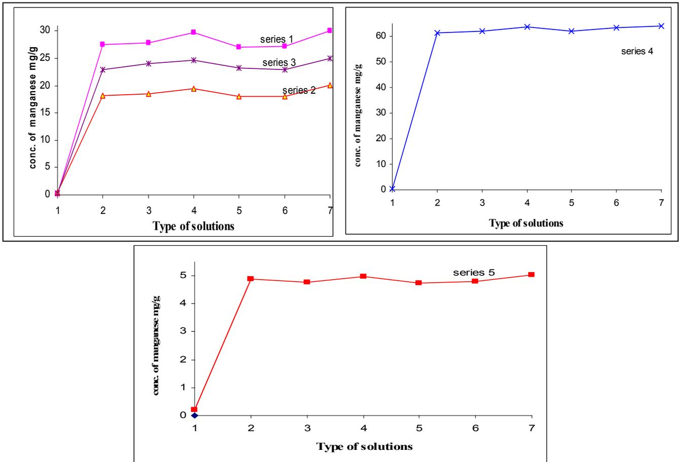
Fig. 1 – Mineralization of samples with different solutions: H<sub>2</sub>O (1), HNO<sub>3</sub> conc. (2), HCl 6 M (3), HNO<sub>3</sub> conc. and HCl 6 M (4), HNO<sub>3</sub> conc. and H<sub>2</sub>O<sub>2</sub> (5), HCl 6M and H<sub>2</sub>O<sub>2</sub> (6), HCl 6 M, HNO<sub>3</sub> conc. and H<sub>2</sub>O<sub>2</sub> (7).
