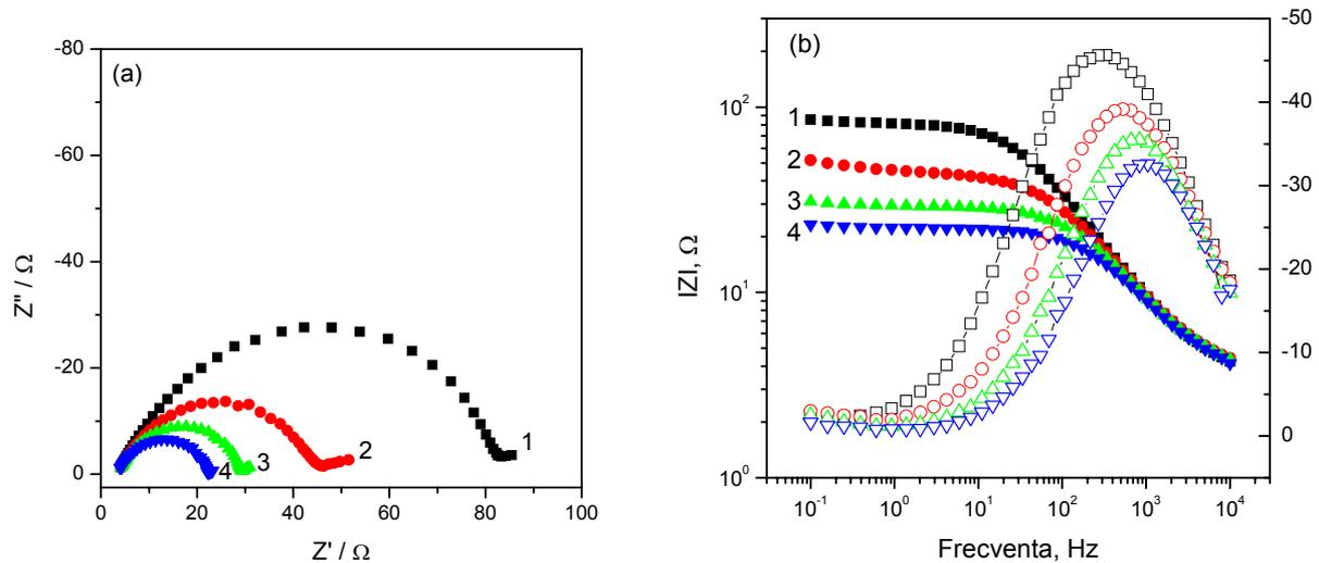
Fig. 2 – Experimental impedance spectra of 18Cr-10Ni stainless steel electrode in artificial seawater as Nyquist plot (a) and Bode plot (b) at various potentials within Tafel region of the HER (V vs. SCE):
