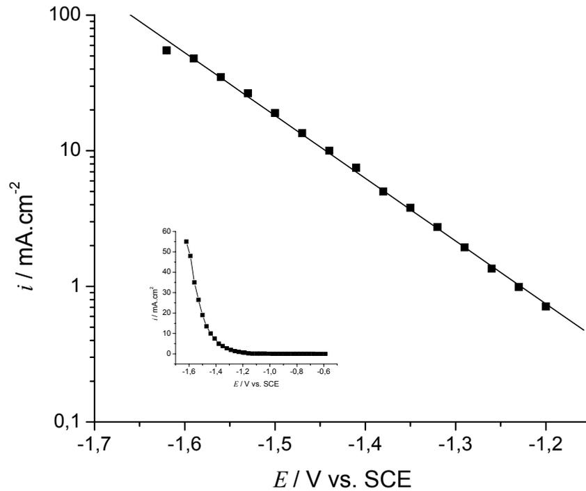
Fig. 1 – Tafel line for the HER on an 18Cr-10Ni stainless steel in artificial seawater, at 295 K. Insert: the polarisation curve on extended potential range.
