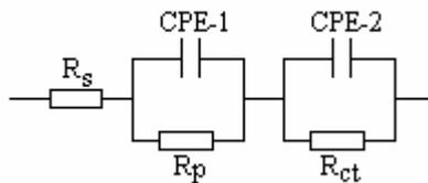
Fig. 3 – Equivalent circuit for NLS fit of the impedance data:  $R_s$  – resistance of the solution;  $R_p$  – pseudo-resistance;  $R_{ct}$  – charge transfer resistance; CPE-1 and CPE-2 – constant phase elements corresponding to pseudo-capacitance ( $C_p$ ) and double layer capacitance ( $C_{dl}$ ), respectively.
