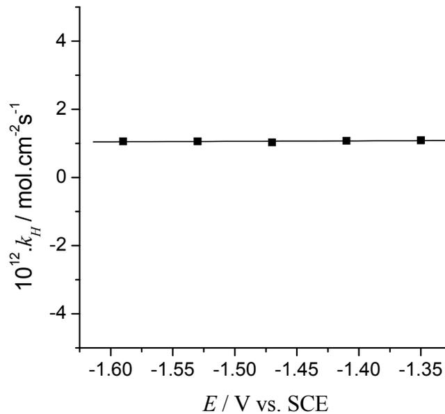
Fig. 6 – Variation with the potential of the chemical rate constant of Heyrowsky step ( $k_H$ ) for the HER on 18Cr-10Ni stainless steel in artificial seawater at 295 K
