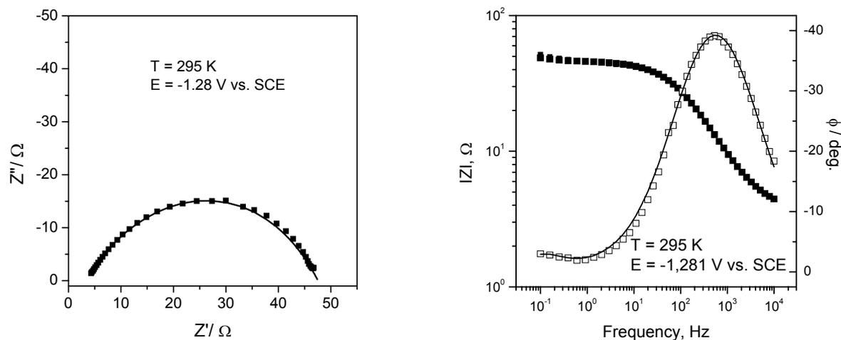
Fig. 4 – The theoretical (as solid curves) and the experimental data (as symbols) impedance spectra in Nyquist (a) and Bode forms (b) obtained from NLS fit results for the HER on an 18Cr-10Ni stainless steel in artificial seawater at 295 K and constant potential (-1.281 V vs. SCE).
