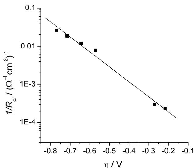
Fig. 5 – Dependence of the charge transfer resistance inverse ( $1/R_{ct}$ ) on overpotential for the HER on 18Cr-10Ni stainless steel electrode in artificial seawater at 295 K.
