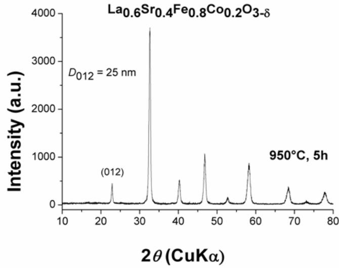
Fig. 1 – XRD patterns of LSFC powder obtained at 950°C, 5h.
