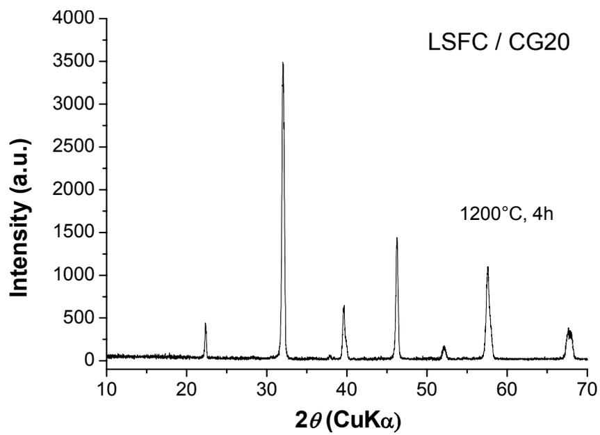
Fig. 5 – XRD patterns of LSFC deposited on CG20 ceramic pellet treated at 1200°C, 4h.
