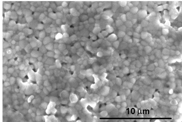
Fig. 4 – SEM picture of CG20 pellet sintered at 1400°C, 4h.
