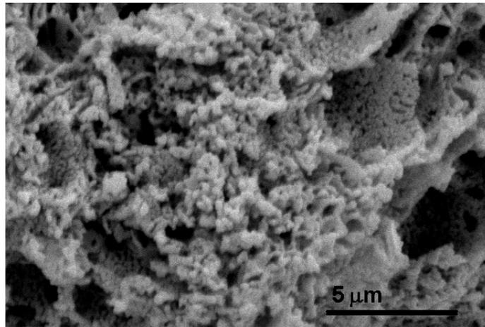
Fig. 2 – SEM micrograph of LSFC powder obtained at 950°C, 5h.
