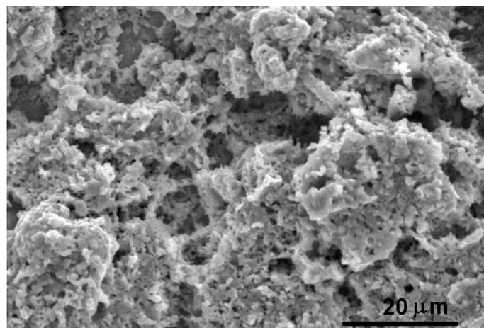
Fig. 6 – SEM micrograph of LSFC deposited on CG20 ceramic pellet treated at 1200°C, 4h.
