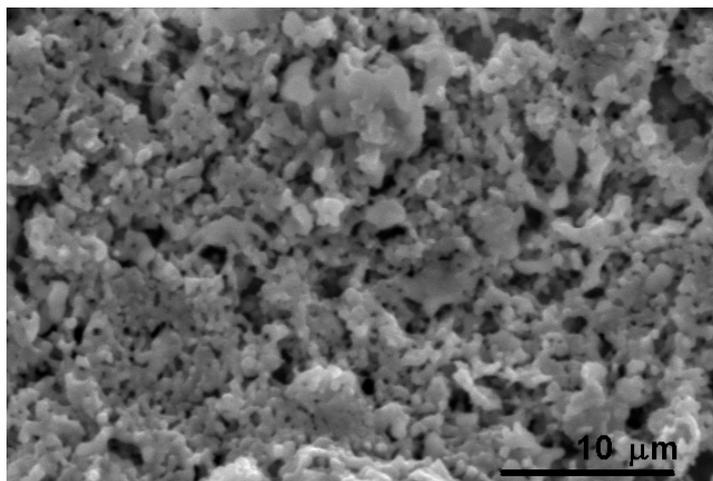
Fig. 8 – SEM micrograph of LSFC-CG20 composite deposited on CG20 ceramic pellet treated at 1200°C, 4h.
