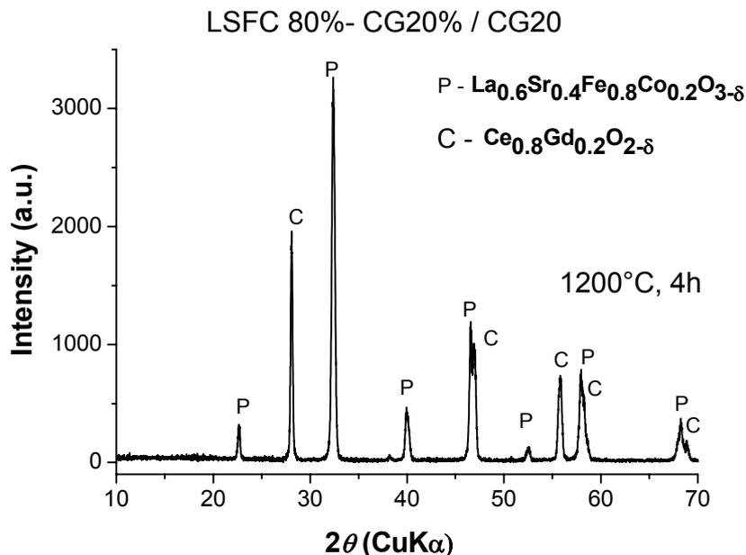
Fig. 7 – XRD patterns of LSFC-CG20 composite deposited on CG20 ceramic pellet treated at 1200°C, 4h.
