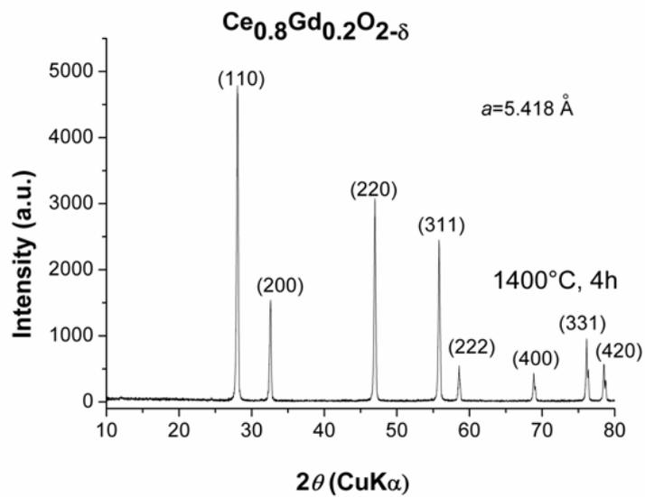
Fig. 3 – XRD patterns of CG20 ceramic pellet sintered at 1400°C, 4h.
