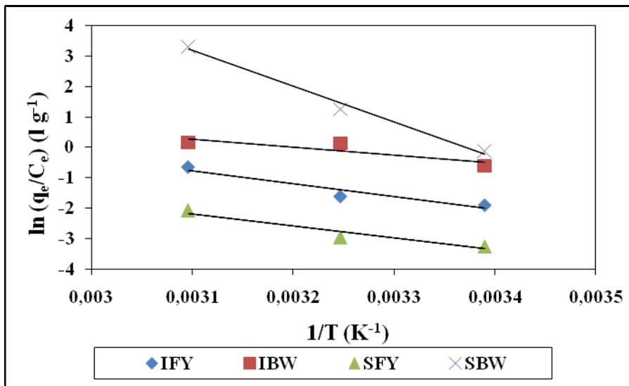
Fig. 6 – Plot of lnK<sub>d</sub> vs 1/T for the estimation of the thermodynamic parameters for Cd(II) biosorption onto SBW, IBW, SFY, and IFY.
