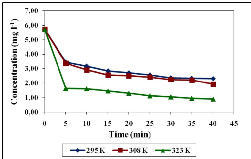
Fig. 2 – Effect of contact time and temperature (295, 308, 323 K) on Cd<sup>2+</sup> concentration during the biosorption process for IFY biosorbent.
