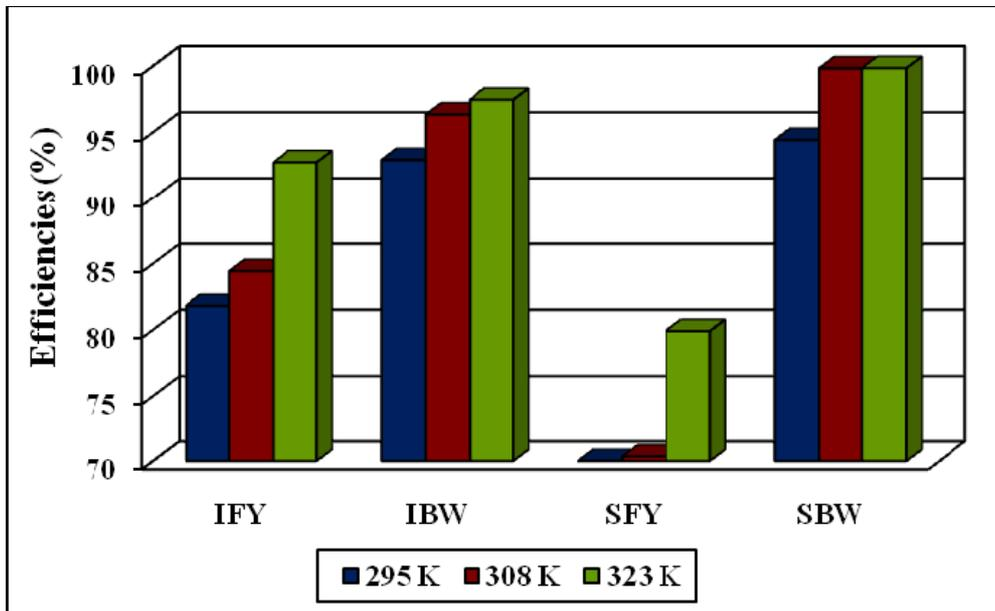
Fig. 3 – Effect of temperature on the maximum removal efficiencies (E,%) of Cd<sup>2+</sup> onto SBW, IBW, SFY, and IFY biosorbents.
