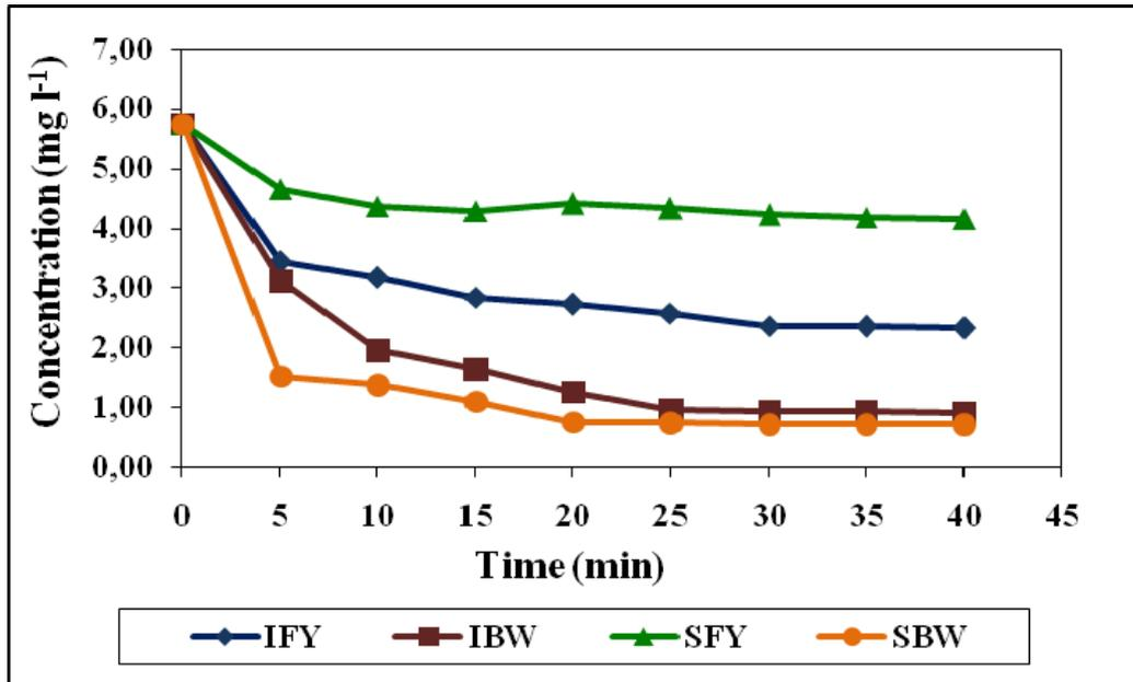
Fig. 1 – Effect of contact time on Cd<sup>2+</sup> concentration during the biosorption process for SBW, IBW, SFY and IFY biosorbents at constant temperature (295 K).
