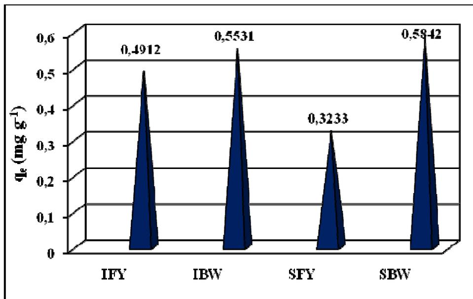
Fig. 4 – Effect of biosorbent type over the adsorption capacity values ( $q_e$ , mg Cd<sup>2+</sup> g<sup>-1</sup>) at constant temperature (323 K).
