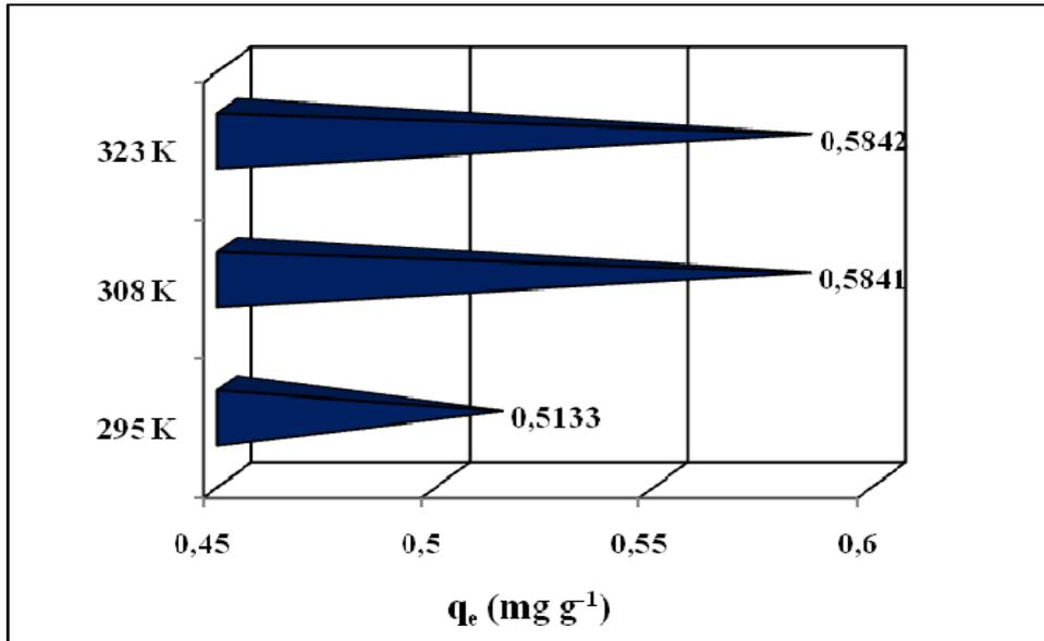
Fig. 5 – Effect of temperature on the adsorption capacity values (q<sub>e</sub>, mg Cd<sup>2+</sup> g<sup>-1</sup>) for SBW biosorbent.
