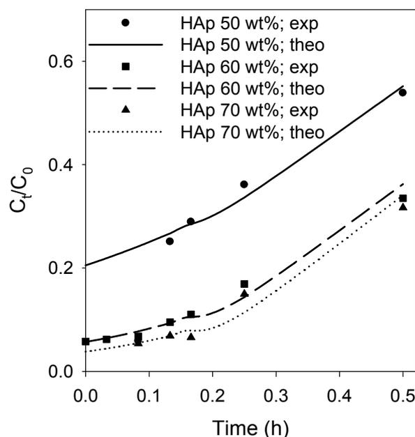
Fig. 4 – Comparison of breakthrough curves between the experimental data and the model fit at different HAp amounts.
