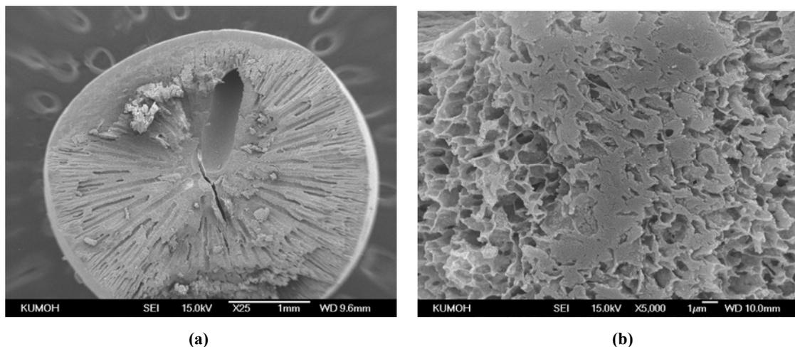
Fig. 1 – SEM micrograph of PAN/HAp composite bead: (a) low magnification; (b) high magnification.
