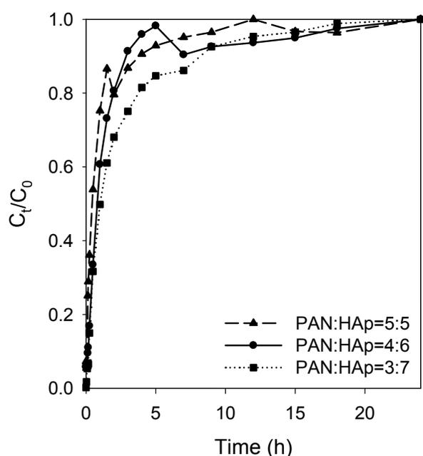
Fig. 3 – Breakthrough curves at different HAp amounts.
