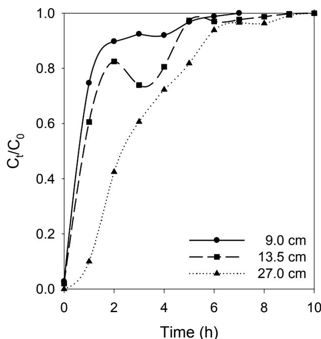
Fig. 2 – Breakthrough curves at different bed heights.
