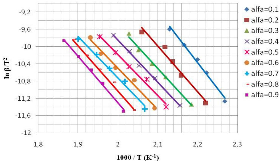
Fig. 5 – The Kissinger–Akahira–Sunose diagrams for ibuprofen at different conversion degrees.
