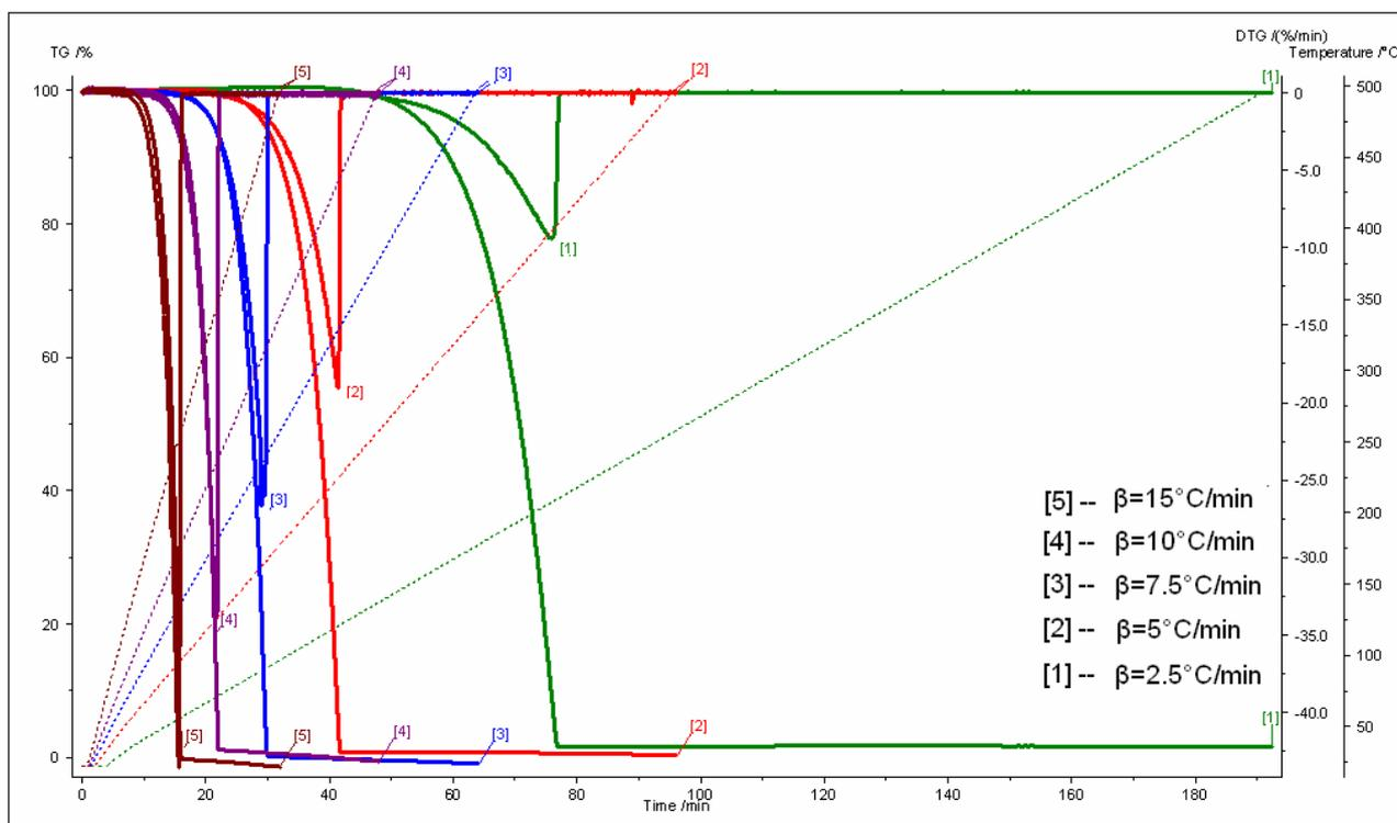
Fig. 1 – The TG/DTG curves of the ibuprofen in nitrogen at different heating rates.
