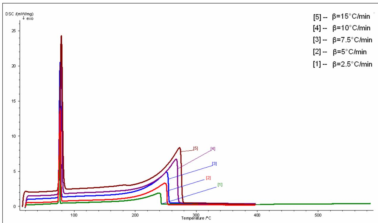
Fig. 2 – The DSC curves of the ibuprofen in nitrogen at different heating rates.
