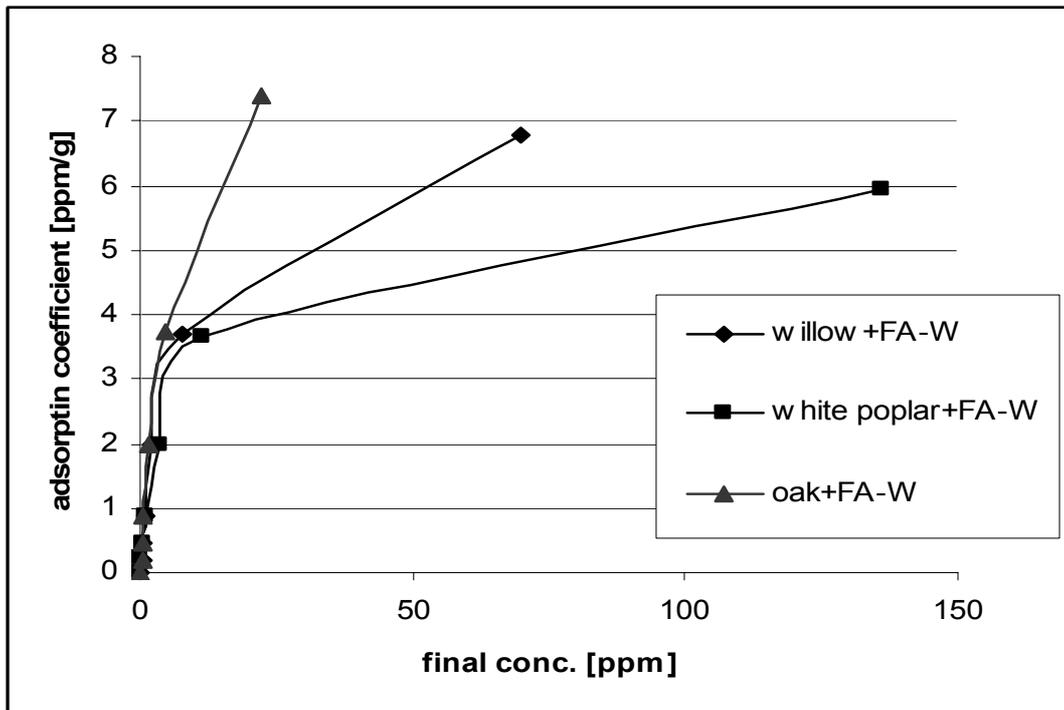
Fig. 6 – Adsorption isotherm of copper on sawdust: FA-W.
