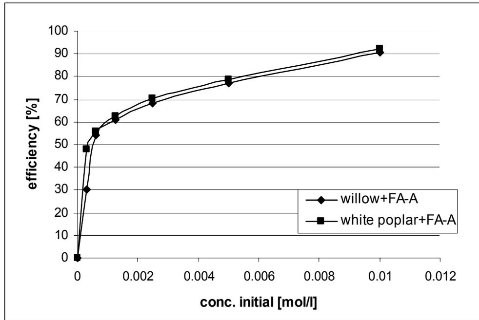
Fig. 5 – Influence of Cu(II) concentration on the adsorption efficiency on Sawdust: FA-A = 1:1.
