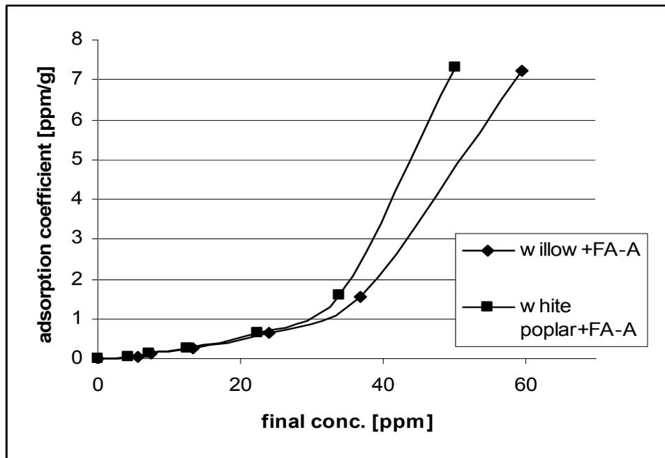
Fig. 7 – Adsorption isotherm of copper on sawdust: FA-A .
