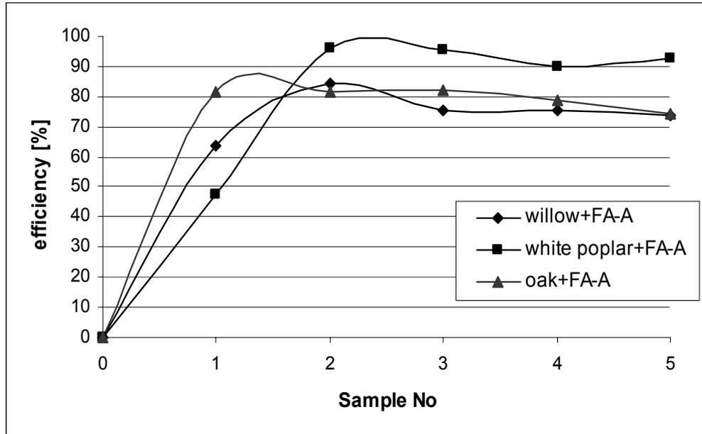
Fig. 2 – Effect of the ratio sawdust: alkali modified fly ash on Cu (II) sorption.
