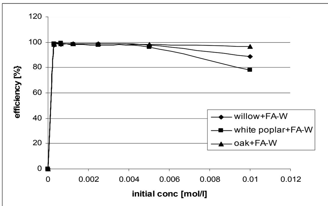
Fig. 4 – Influence of Cu(II) concentration on the adsorption efficiency on Sawdust: FA-W = 1:1.
