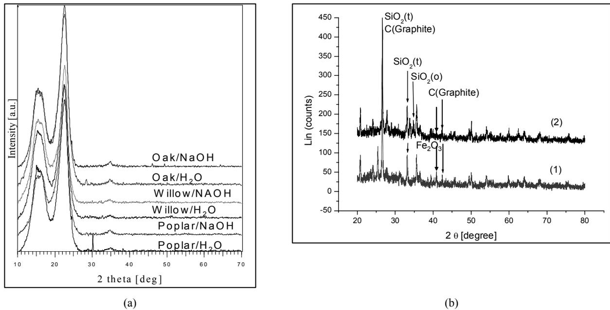
Fig. 1 – XRD diffraction patterns for wood (a) and fly ash (b).
