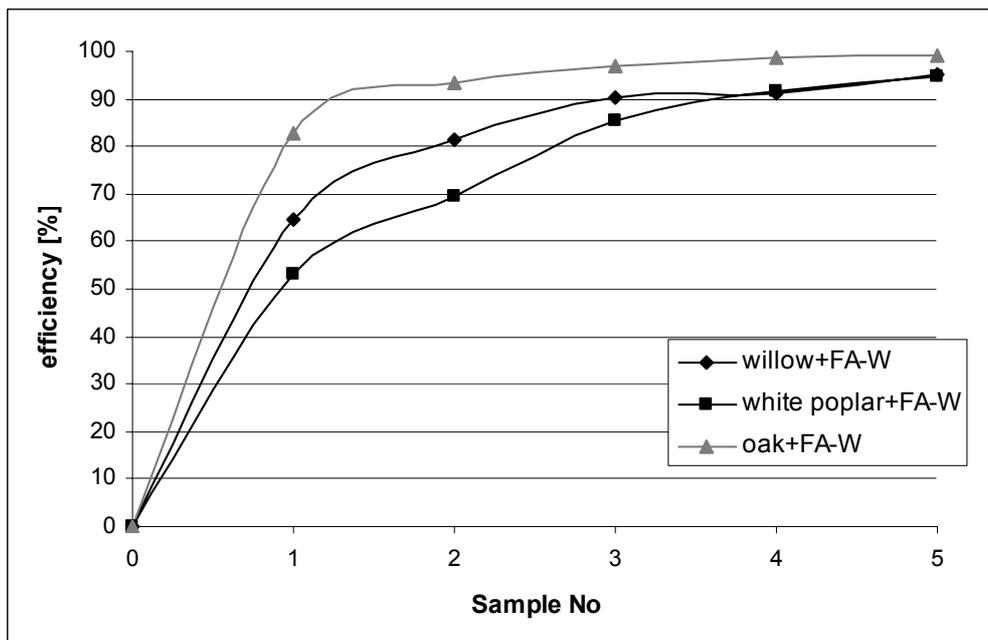
Fig. 3 – Effect of the ratio sawdust: fly ash washed with distilled on Cu(II) sorption.
