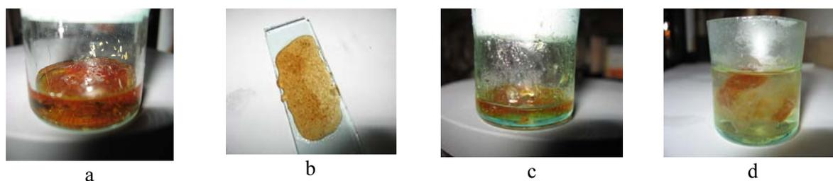
Fig. 2 – Photographs of dissolution of beech sawdust (a, b), respectively beech cellulose (c, d) in ionic liquid.
