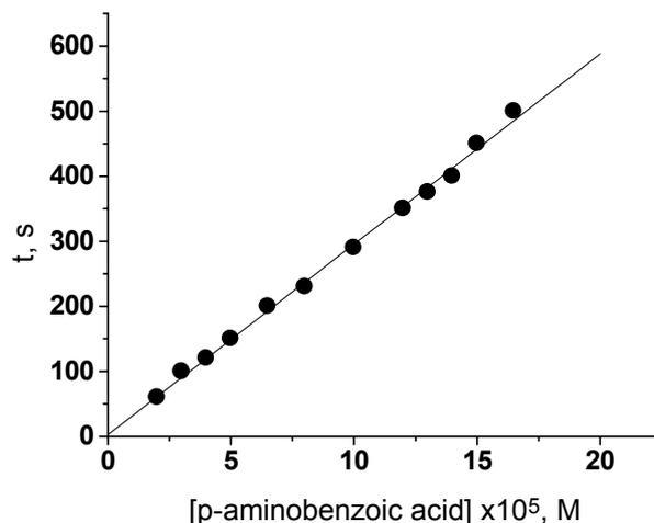
Fig. 5 – Linear calibration curve for p-aminobenzoic acid.
