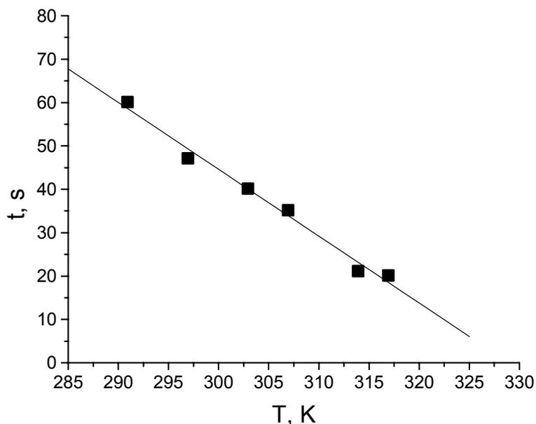
Fig. 4 – Dependence of bromine generation time to temperature in the case of:
