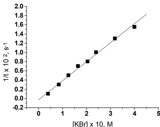
Fig. 2 – Dependence of bromine generation time to KBr in the case of: [p-aminobenzoic acid] =  $8 \cdot 10^{-5}$  M,  $[H^+] = 2 \cdot 10^{-2}$  M,  $[KBrO_3] = 3 \cdot 10^{-3}$  M, at  $T = 293$  K.
