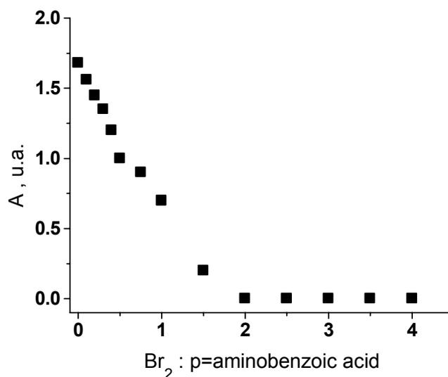
Fig. 1 – Stoichiometry of the bromination reaction of p-amino benzoic acid (Absorbance vs. Br<sub>2</sub>: p-aminobenzoic acid).
