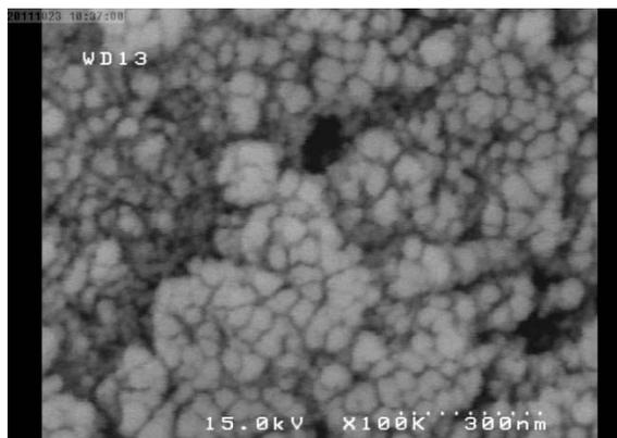
Fig. 1 – The SEM image of  $\gamma$ - $\text{Al}_2\text{O}_3$  nanoparticles.
