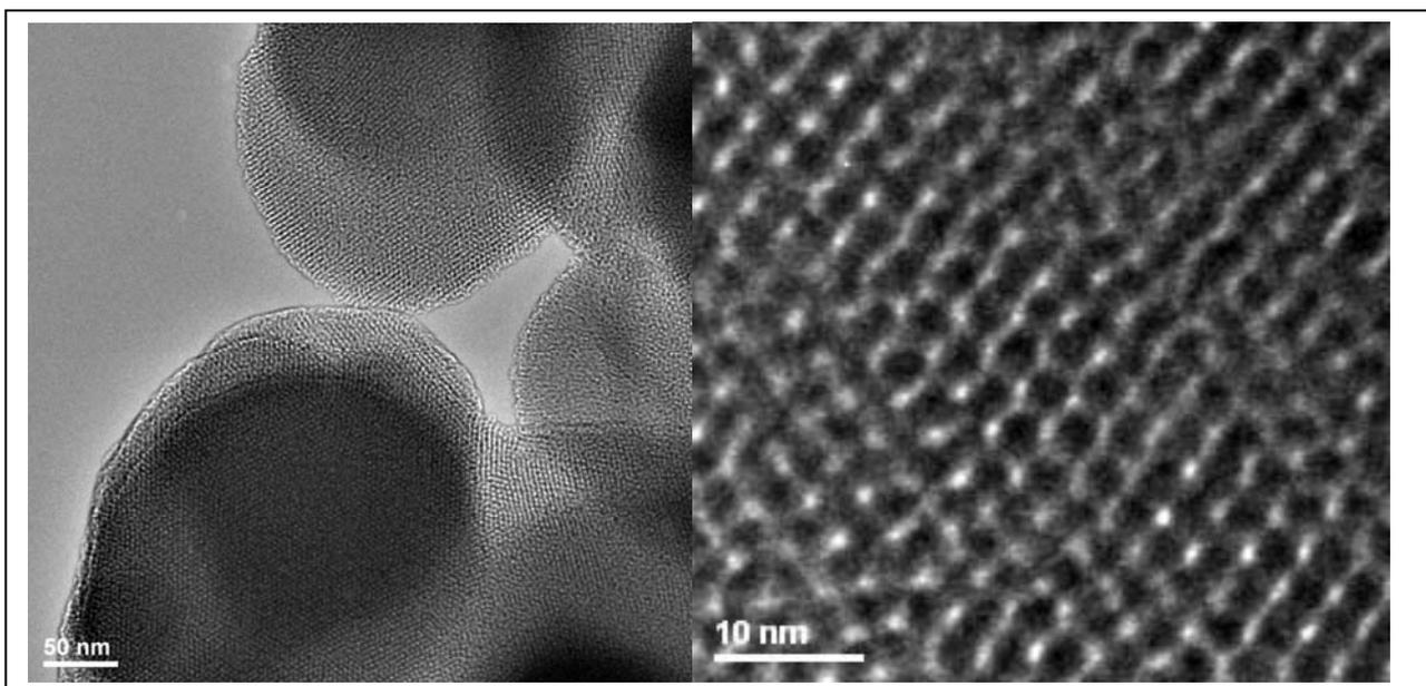
Fig. 2 – HR-TEM analysis of the MCM-41 sample (overall image left-hand side, and detailed image right-hand side).
