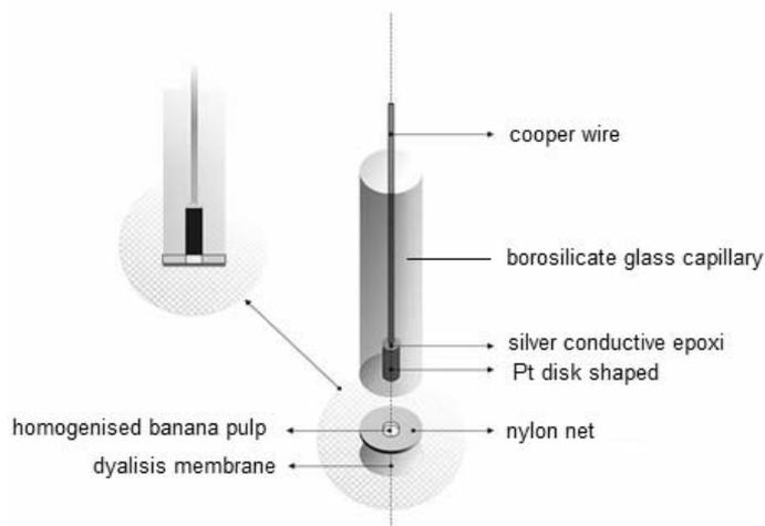
Fig. 6 – The sketch of the construction of the “bananatrode”.
