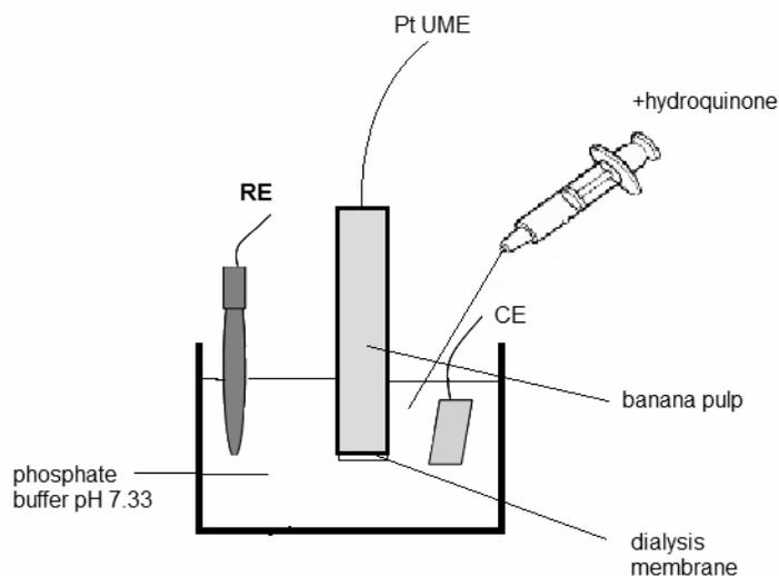
Fig. 5 – The experimental setup used in SECM experiments.
