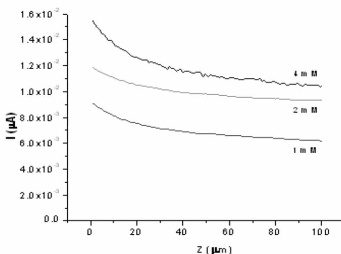
Fig. 1 –  $H_2Q$  concentration profiles for different initial  $H_2Q$  concentrations. Applied electrode potential for Pt UME was + 400 mV vs. Ag quasi-reference electrode.
