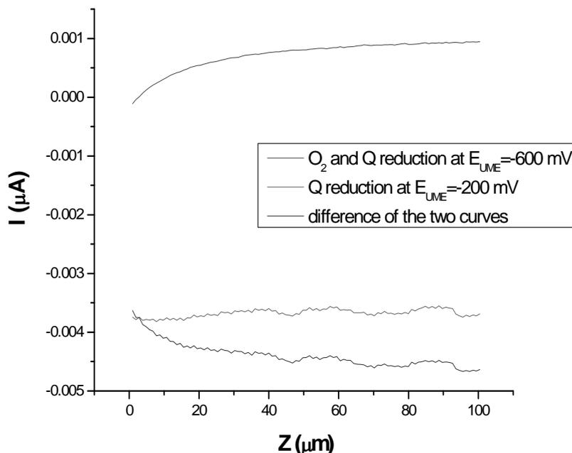
Fig. 3 – The current-distance (approaching) curves for 1 mM H<sub>2</sub>Q in PBS of pH 7.33 at two different working electrode potentials: -0.6 V (simultaneous reduction of O<sub>2</sub> and H<sub>2</sub>Q) and at -0.2 V (reduction of O<sub>2</sub> only) and their difference.
