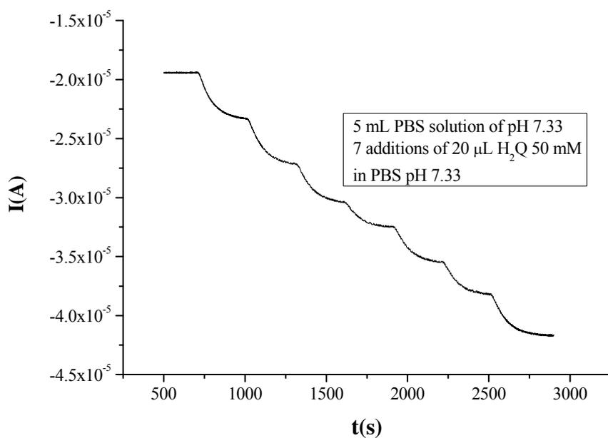
Fig. 4 – The current-time responses for one (20  $\mu\text{L}$   $\text{H}_2\text{Q}$  50 mM in PBS of pH 7.33) of the four series of seven constant-volume additions.
