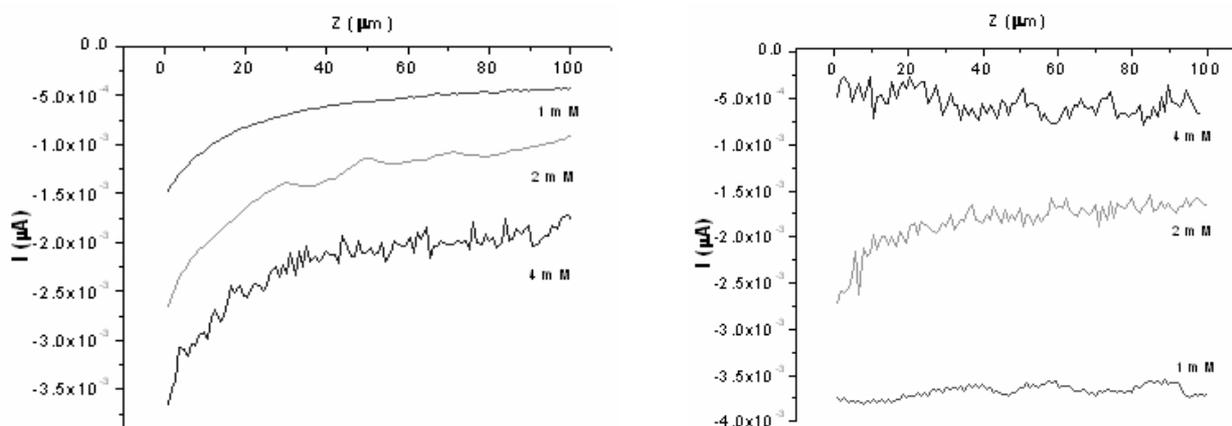
Fig. 2 – The current-distance (approaching) curves for the three different  $H_2Q$  concentrations in PBS of pH 7.33 at -0.2 V (A) and -0.6V (B) working electrode potential.
