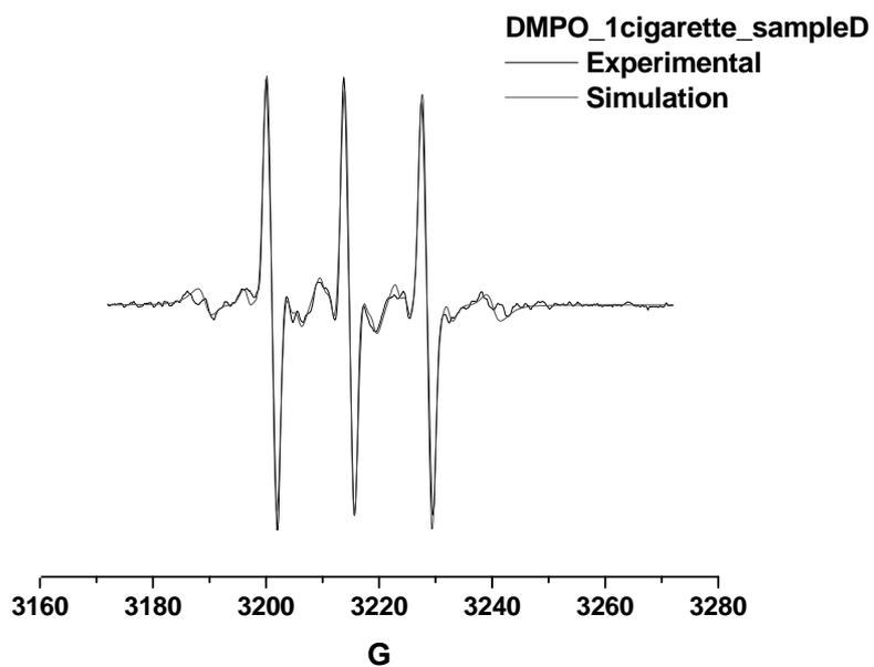
Fig. 5 – EPR spectrum for a whole type D cigarette obtained with the DMPO spin-trap.
