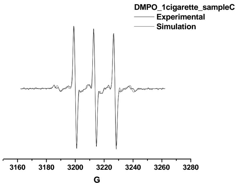
Fig. 4 – EPR spectrum corresponding to DMPO adducts obtained after consumption of a whole type C cigarette.
