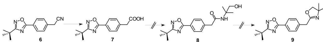
Scheme 5 – Proposed synthetic route for 3-*tert*-butyl-5-[4-((4,4-dimethyl-4,5-dihydrooxazol-2-yl)methyl)phenyl]-1,2,4-oxadiazole (**9**).
