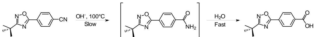
Scheme 3 – Hydrolysis of 4-[3-(*tert*-butyl)-1,2,4-oxadiazol-5-yl]benzonitrile in basic conditions.
