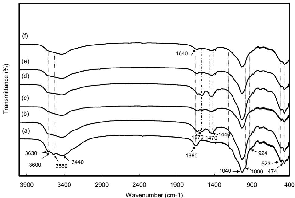
Fig. 2 – FTIR spectra of raw bentonite (a) and samples contain different weight ratio ZnO/bentonite of 0.2 (b) 0.4 (c) 0.6(d) 0.8 (e) and 1 (f).
