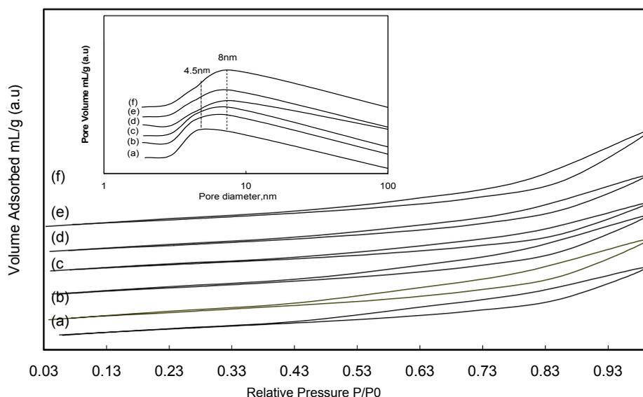
Fig. 4 – Nitrogen adsorption-desorption isotherms and pore size distributions of raw bentonite (a) and samples contain different weight ratio ZnO/bentonite of 0.2 (b) 0.4 (c) 0.6(d) 0.8 (e) and 1 (f).
