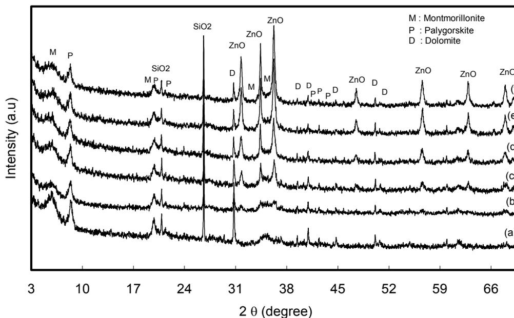
Fig. 1 – X-Ray diffraction patterns of raw bentonite (a) and samples contain different weight ratio ZnO/bentonite of 0.2 (b) 0.4 (c) 0.6 (d) 0.8 (e) and 1(f).
