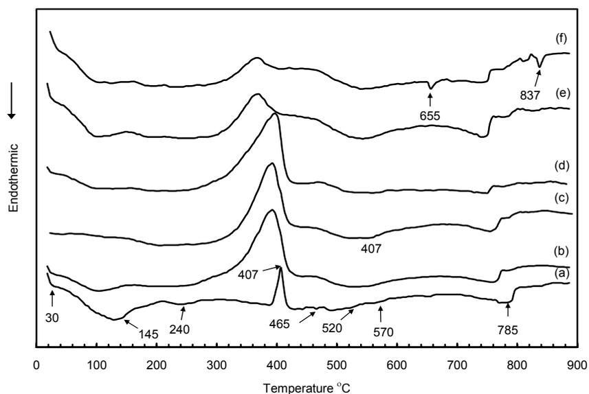
Fig. 3 – DTA curves of raw bentonite (a) and samples contain different weight ratio ZnO/bentonite of 0.2 (b) 0.4 (c) 0.6(d) 0.8 (e) and 1 (f).
