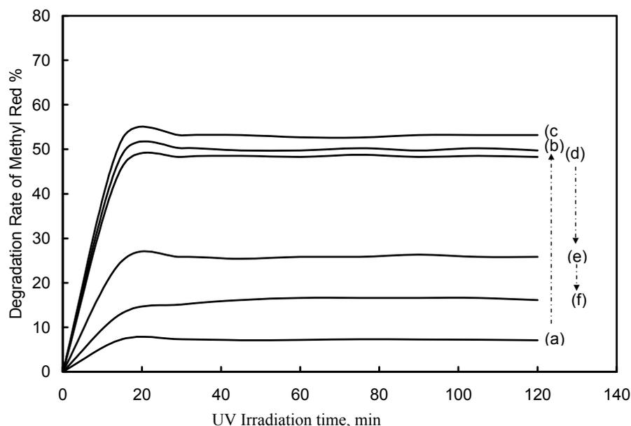
Fig. 5 – Photocatalytic degradation rate of raw bentonite (a) and samples contain different weight ratio ZnO/bentonite of 0.2 (b) 0.4 (c) 0.6(d) 0.8 (e) and 1 (f).
