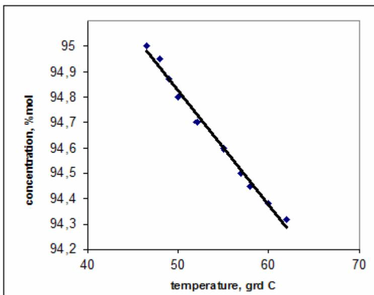
Fig. 3 – Variation of the concentration at the head of the packed column versus the jacket temperature for methanol – ethanol mixture.
