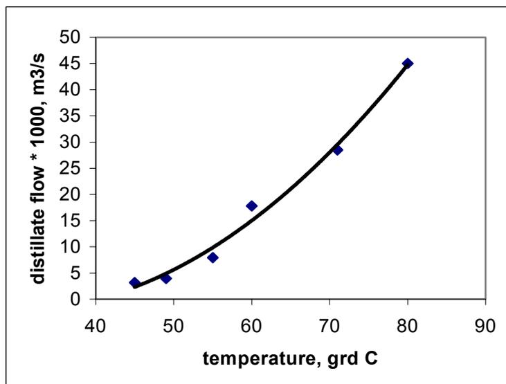
Fig. 2 – Variation of the distillate flow with the jacket temperature in the bubble-cap plate column for benzene – dichlor-ethane mixture.
