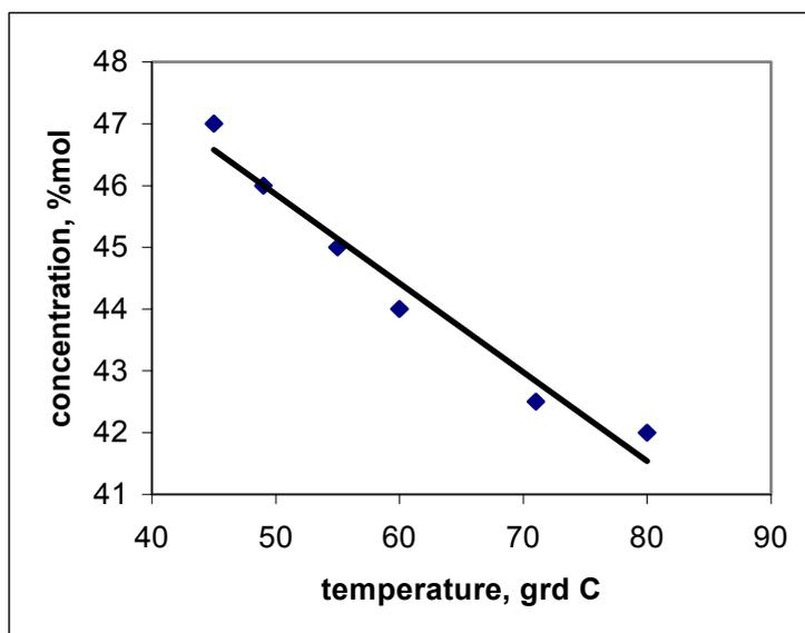
Fig. 1 – Variation of concentration at the head of the bubble-cap plate column versus jacket temperature for benzene – dichlor-ethane mixture.
