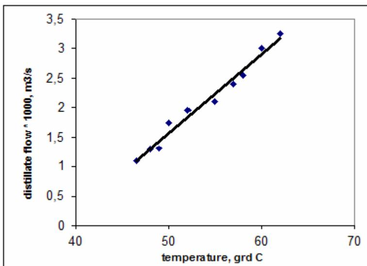
Fig. 4 – Variation distillate flow versus the jacket temperature in the packed column for methanol – ethanol mixture.
