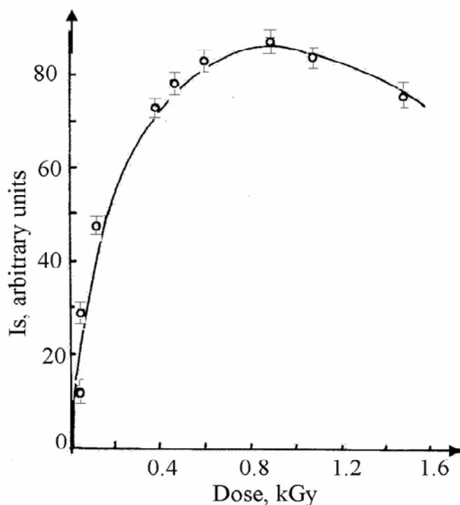
Fig. 3 – Variation of the intensity of the EPR signal (arbitrary units) as a function of irradiation dose.
