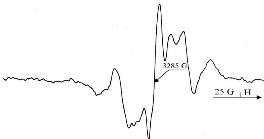
Fig. 2 – The EPR spectrum of  $\beta\text{Ala-LHis}$  irradiated with a 2 kGy dose.
