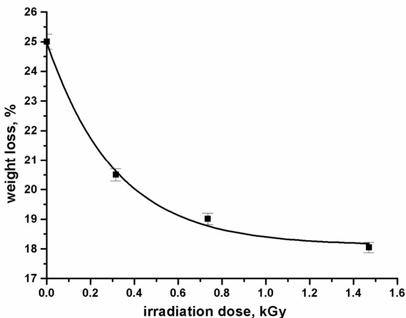
Fig. 7 – Dependence of the weight loss of L-alanyl-glycine on heating to  $240^\circ\text{C}$ , on irradiation dose (kGy).
