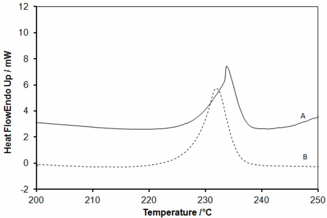
Fig. 4 – DSC thermograms of L-alanyl-glycine (L Ala-Gly) (A)- non-irradiated and (B)-3h- irradiated (0.315 kGy).
