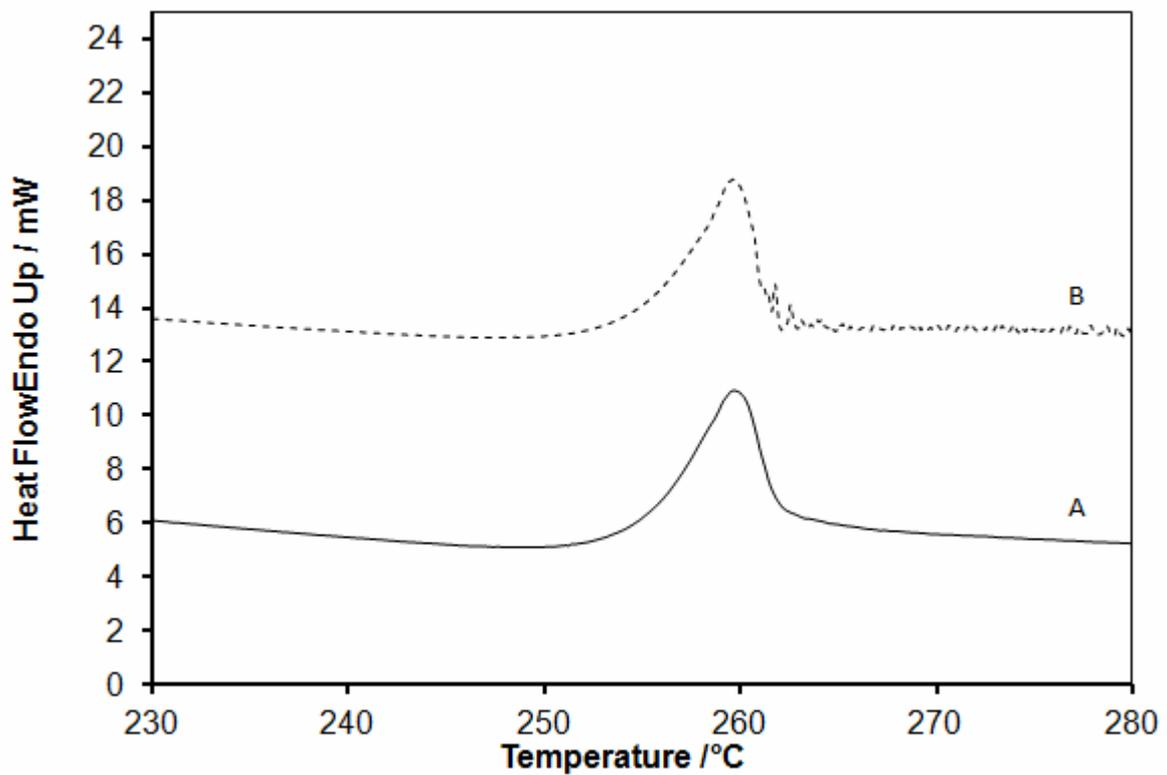
Fig. 5 – DSC thermograms of carnosine (A)- non-irradiated and (B)-3h- irradiated (0.315 kGy).
