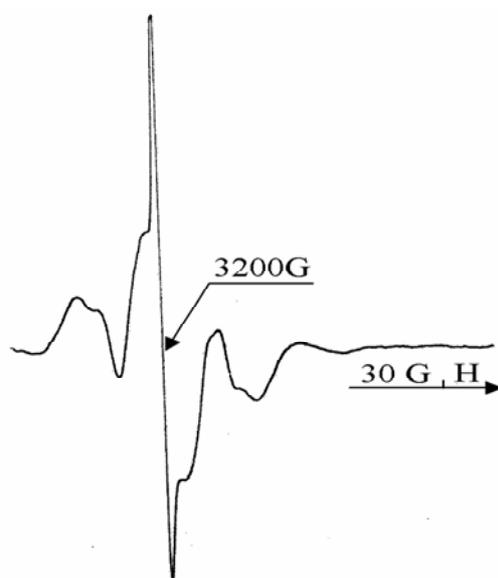
Fig. 1 – The EPR spectrum of  $L\text{Ala-Gly}$  irradiated with a 2 kGy dose.
