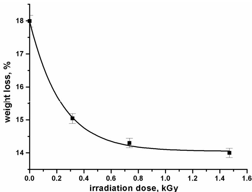
Fig. 8 – Dependence of the weight loss of carnosine on heating to 270<sup>0</sup>C, on irradiation dose (kGy).
