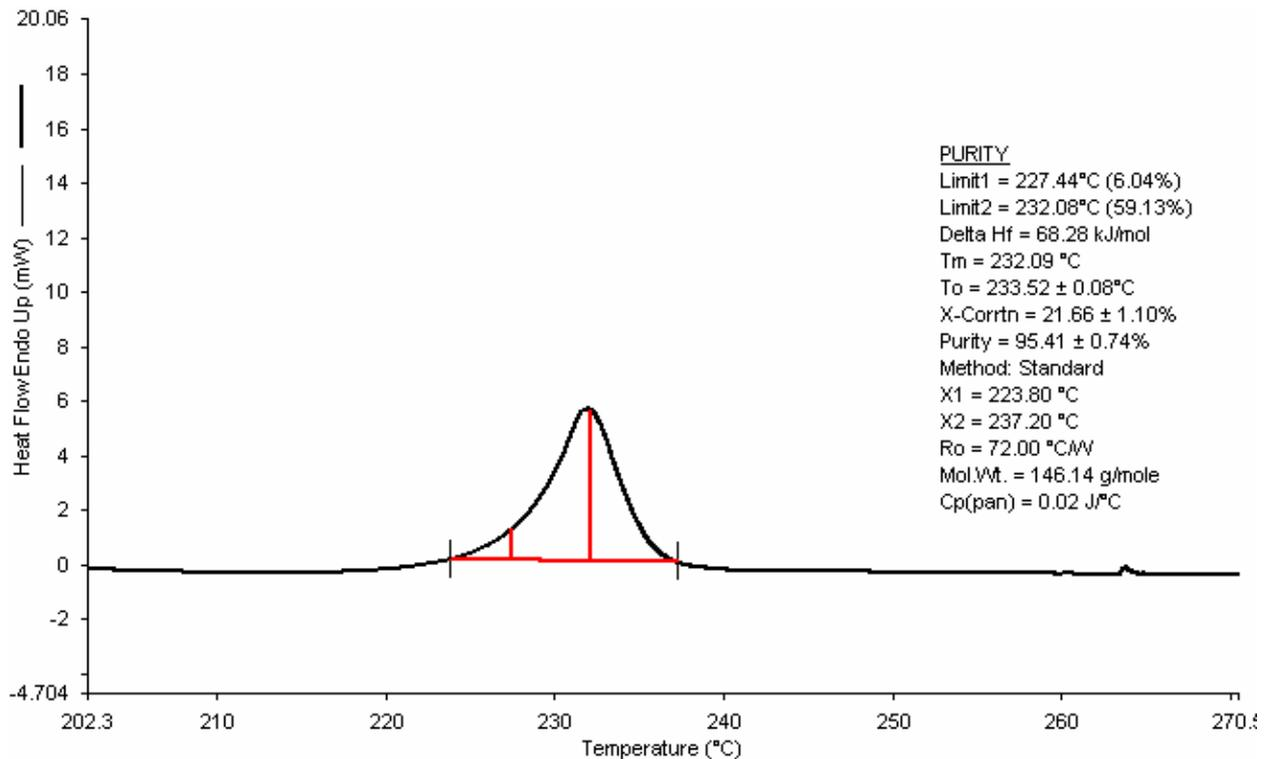
Fig. 9 – Determination of purity using Pyris software for L-alanyl-glycine 3h-irradiated (0.31 kGy).
