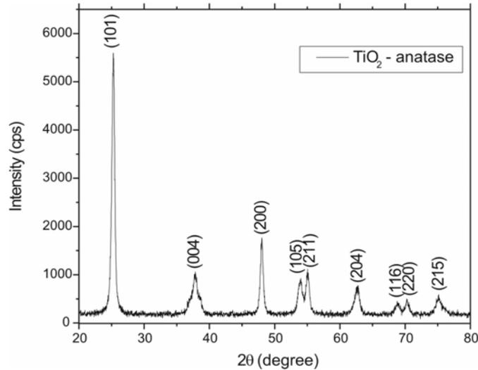
Fig. 2 – XRD spectrum of TiO<sub>2</sub> sample.
