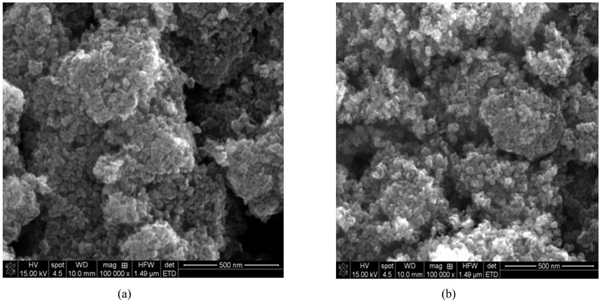
Fig. 3 – SEM images of TiO<sub>2</sub> powder (a) before and (b) after testing with CO.
