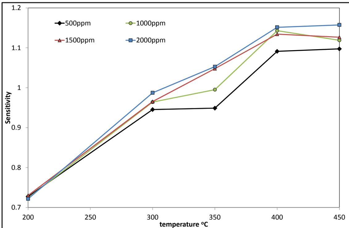
Fig. 4 – Electrical response of TiO<sub>2</sub> powder for various concentrations of CO depending on temperature.
