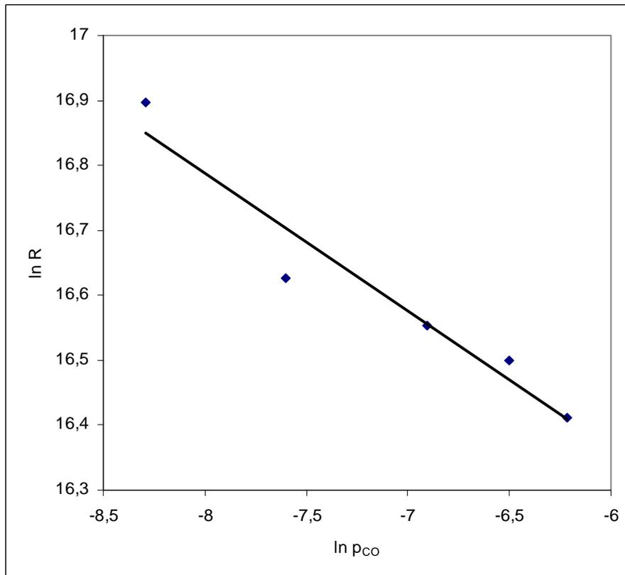
Fig. 6 – Arrhenius plot of electrical resistance as a function of partial pressure of CO.
