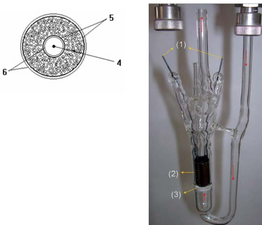
Fig. 1 – The reaction cell with: (1) Tungsten wires, (2) Coaxial tantalum electrodes (cylinder type), (3) Ceramic frit, (4) Thermocouple (slice view), (5) Coaxial tantalum electrodes (slice view), (6) Glass walls (slice view).
