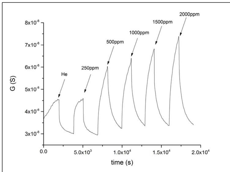
Fig. 5 – Electric response of TiO<sub>2</sub> sample at 400°C, for different CO concentration.
