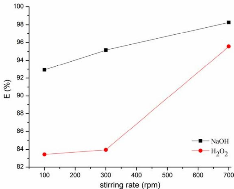
Fig. 3 – The effect of stirring rate over the removal efficiency for Cd (II) treated fir tree sawdust on Cd (II) adsorption;  $C_i = 50$  mg/L, 5 g biomass,  $d = 0.4-0.6$  mm, 296 K, pH 5.5.
