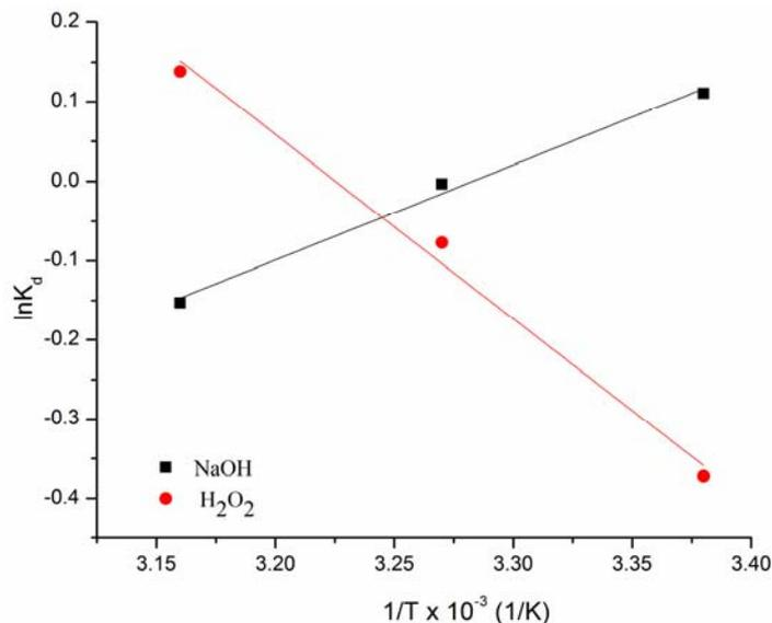
Fig. 5 – Plot of  $\ln K_d$  versus  $1/T$  for the estimation of the thermodynamic parameters for Cd (II) adsorption on fir tree treated sawdust.
