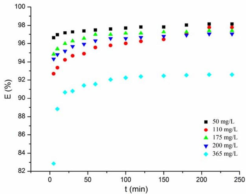
Fig. 2 – The effect of contact time over the removal efficiency for Cd (II) adsorption on NaOH treated fir tree sawdust on Cd (II) adsorption;  $C_i = 50\text{-}365$  mg/L, 5 g biomass,  $d = 0.4\text{-}0.6$  mm, 296 K, pH 5.5, 700 rpm.
