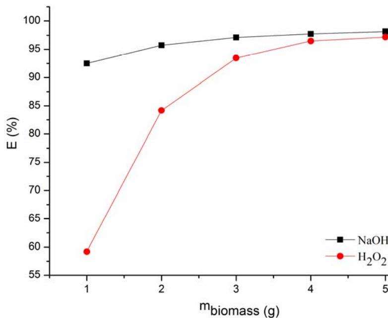
Fig. 4 – The effect of the biomass quantity on Cd (II) removal efficiency;  $C_i = 50$  mg/L,  $d = 0.4-0.6$  mm, 296 K, pH 5.5, 700 rpm.
