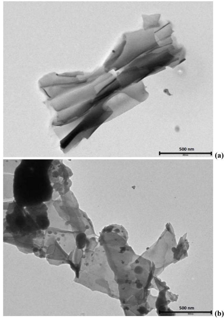
Fig. 1 – TEM images of (a) untreated (8000 $\times$ ) and (b) NaOH (8000 $\times$ ) treated fir tree sawdust.
