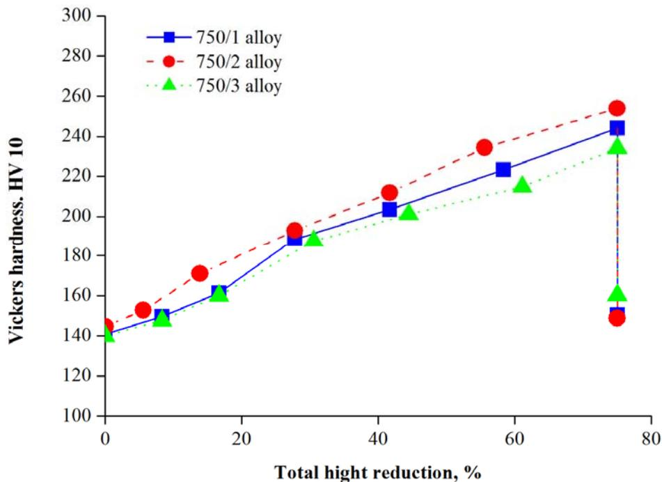
Fig. 2 – Dependence of hardness alloy fineness of 750 on total height reduction.
