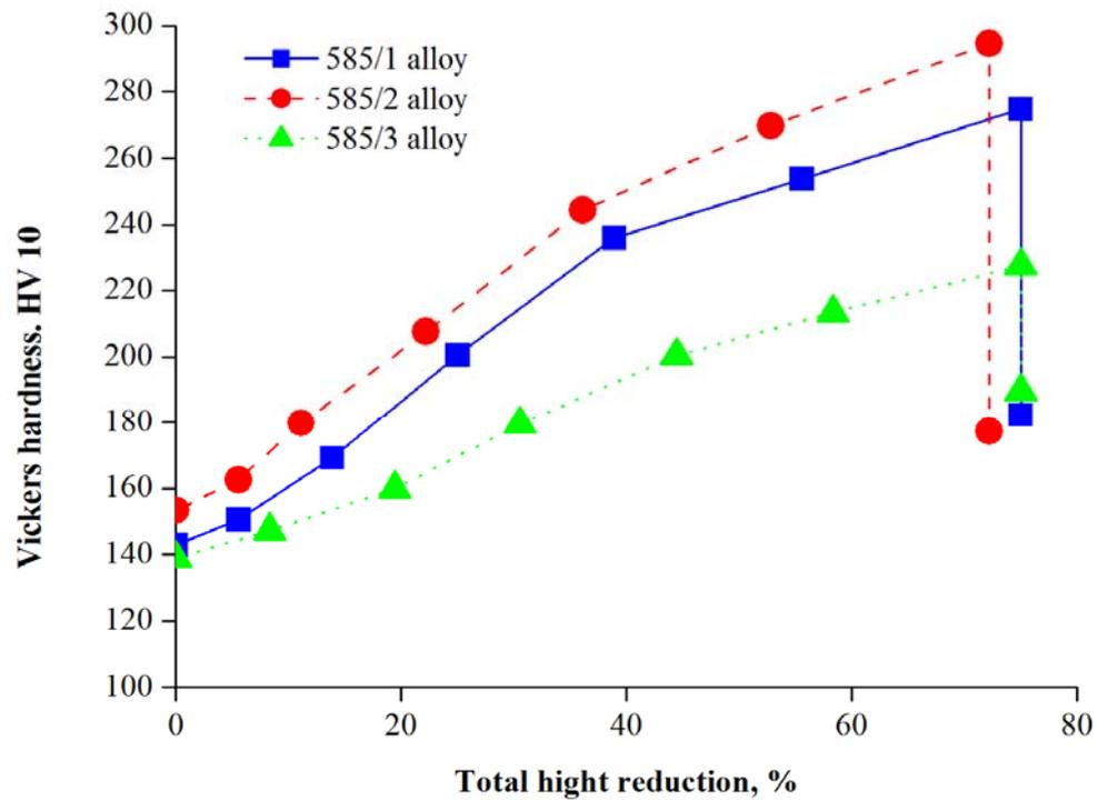
Fig. 1 – Dependence of hardness alloy fineness of 585 on total height reduction.
