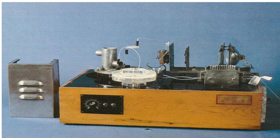
Fig. 3 – Prototype AutoAnalyzer version in 1953. Reproduced from Ref 15.
