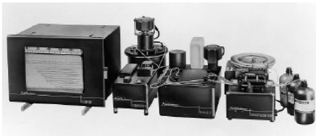
Fig. 4 – First commercial AutoAnalyzer launched in 1957. Reproduced from Ref 15.
