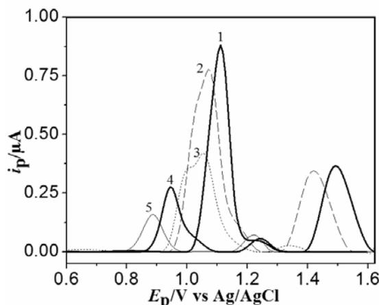
Fig. 1 – DP voltammograms of  $10 \mu\text{g mL}^{-1}$  NLT solution on different pH values as pH 1.5 phosphate buffer (1); pH 2.5 phosphate buffer (2); pH 3.7 acetate buffer (3); pH 5.7 acetate buffer (4); pH 8.0 phosphate buffer (5).
