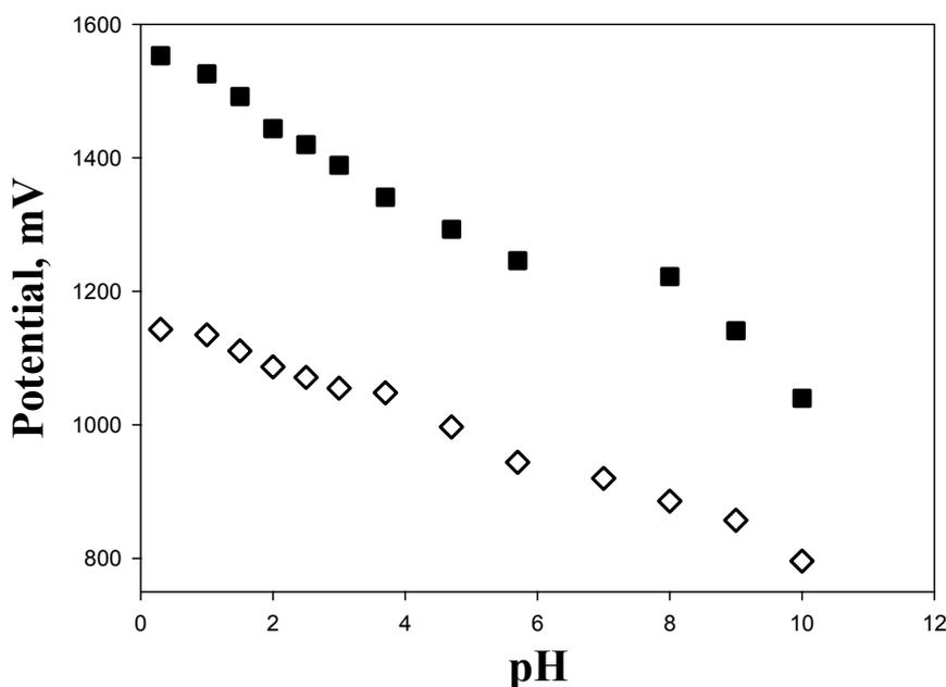
Fig. 2 –  $E_p$ -pH plot of  $10 \mu\text{g mL}^{-1}$  NLT obtained by DPV in various buffer solutions and pH values; the first peak ( $\diamond$ ) and the second peak ( $\blacksquare$ ).
