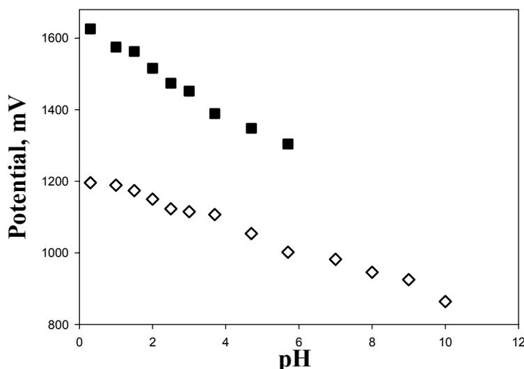
Fig. 4 –  $E_p$ -pH plot of  $10 \mu\text{g mL}^{-1}$  NLT obtained by CV in various buffer solutions and pH values; the first peak ( $\diamond$ ) and the second peak ( $\blacksquare$ ).
