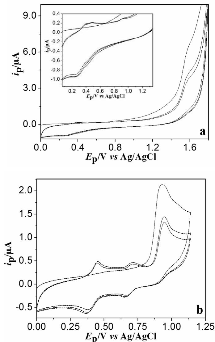
Fig. 5 – By repetitive cyclic voltammograms in 0.1 M H<sub>2</sub>SO<sub>4</sub> 40 ppm lidocaine (a), 20 ppm diclofenac (b) by 100 mV s<sup>-1</sup>.
