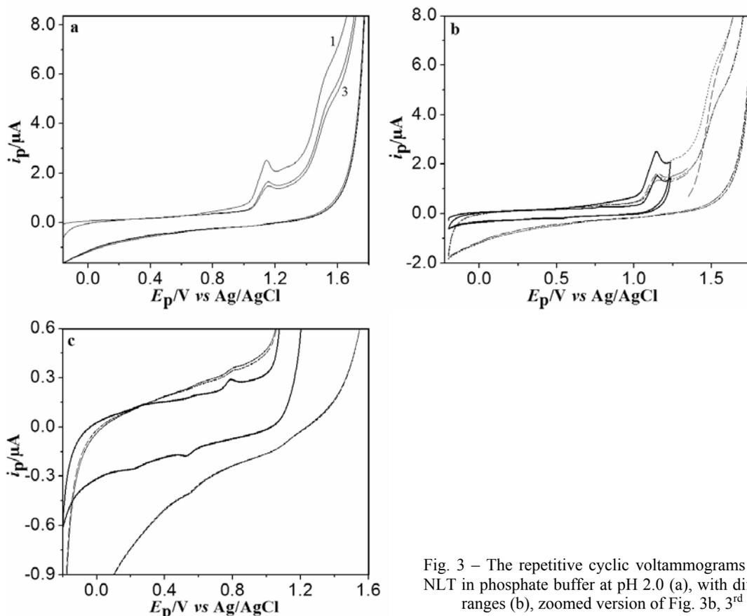
Fig. 3 – The repetitive cyclic voltammograms of  $20 \mu\text{g mL}^{-1}$  NLT in phosphate buffer at pH 2.0 (a), with different potential ranges (b), zoomed version of Fig. 3b, 3<sup>rd</sup> scan (c).
