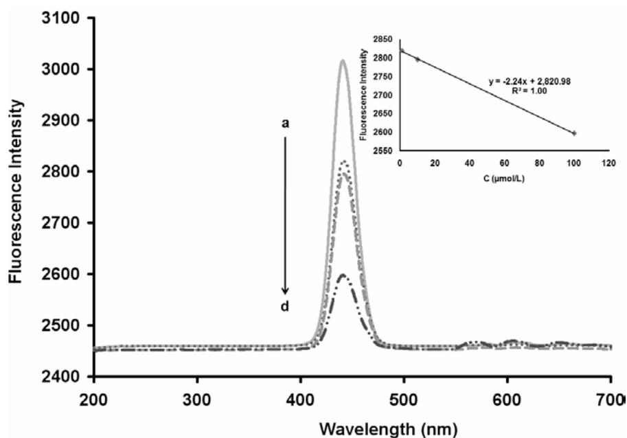
Fig. 6 – Fluorescence quenching of  $\text{KMnO}_4$  upon addition of increasing amount of FA; (a) 0  $\mu\text{mol/L}$ , (b) 1  $\mu\text{mol/L}$ , (c) 10  $\mu\text{mol/L}$ , (d) 100  $\mu\text{mol/L}$ . Inset: Calibration curve of concentration of FA against fluorescence intensity. Conditions:  $[\text{KMnO}_4]$ ,  $10^{-3}$  mol/L; PBS pH = 3.
