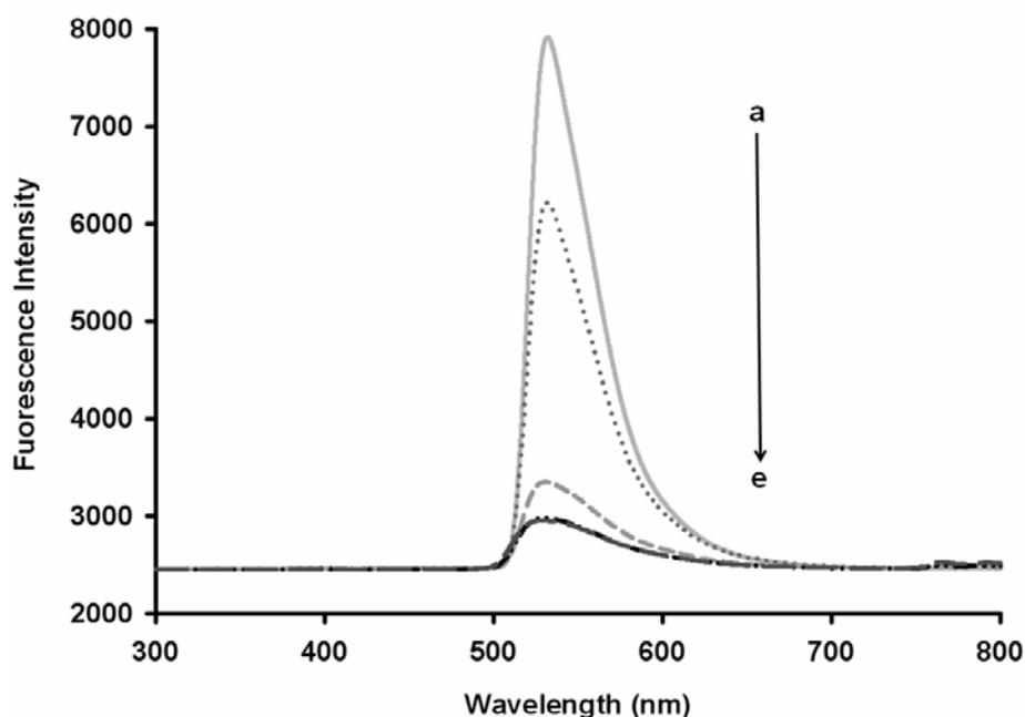
Fig. 1 – Overlay fluorescence spectra of mixed solutions (FA,  $10^{-4}$  mol/L; Fluorescein,  $10^{-3}$  mol/L, PBS); (a) pH = 8, (b) pH = 7, (c) pH = 6, (d) pH = 5 and (e) pH = 4.
