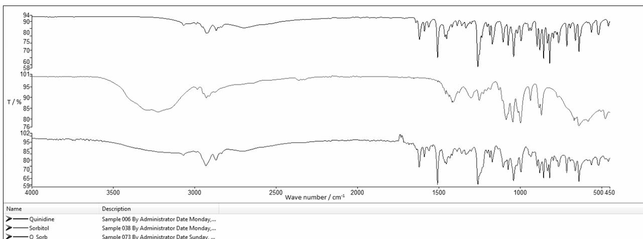
Fig. 2B – FTIR spectra of quinidine, sorbitol and the binary mixture.
