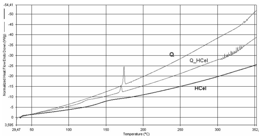
Fig. 3E – DSC curves of quinidine, hydroxyethylcellulose and the binary mixture.
