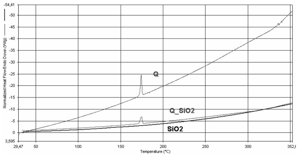
Fig. 3C – DSC curves of quinidine, SiO<sub>2</sub> and the binary mixture.
