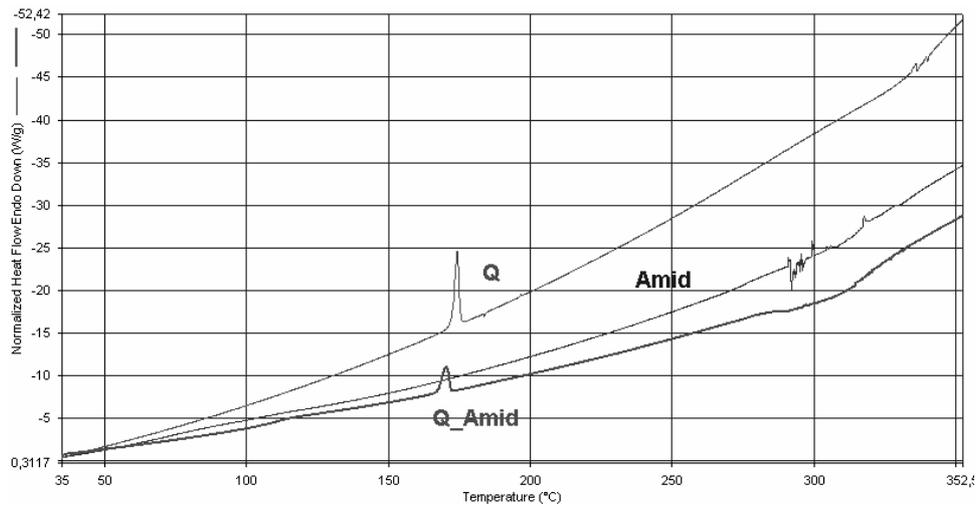
Fig. 3A – DSC curves of quinidine, starch and the binary mixture.
