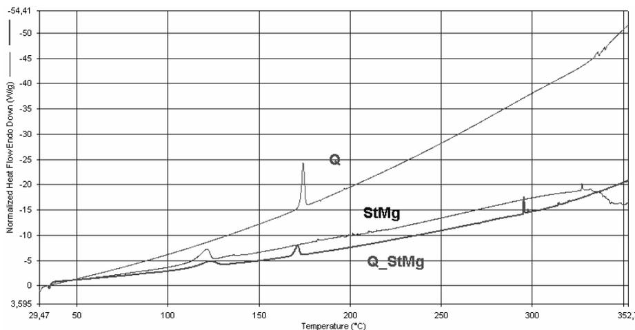
Fig. 3D – DSC curves of quinidine, magnesium stearate and the binary mixture.
