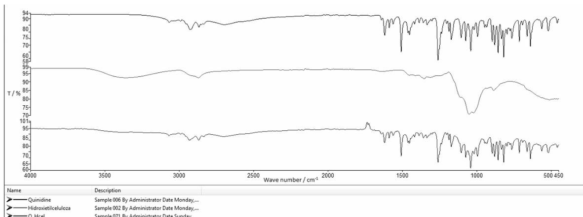
Fig. 2E – FTIR spectra of quinidine, hydroxyethylcellulose and the binary mixture.
