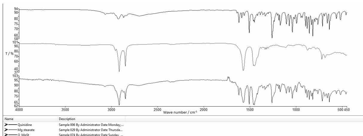
Fig. 2D – FTIR spectra of quinidine, magnesium stearate and the binary mixture.
