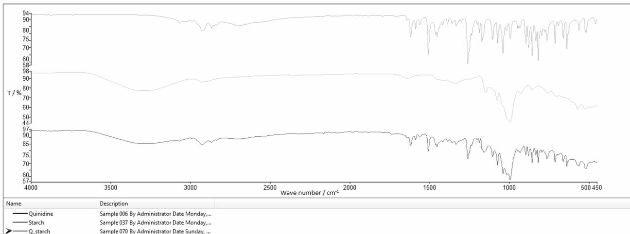
Fig. 2A – FTIR spectra of quinidine, starch and the binary mixture.
