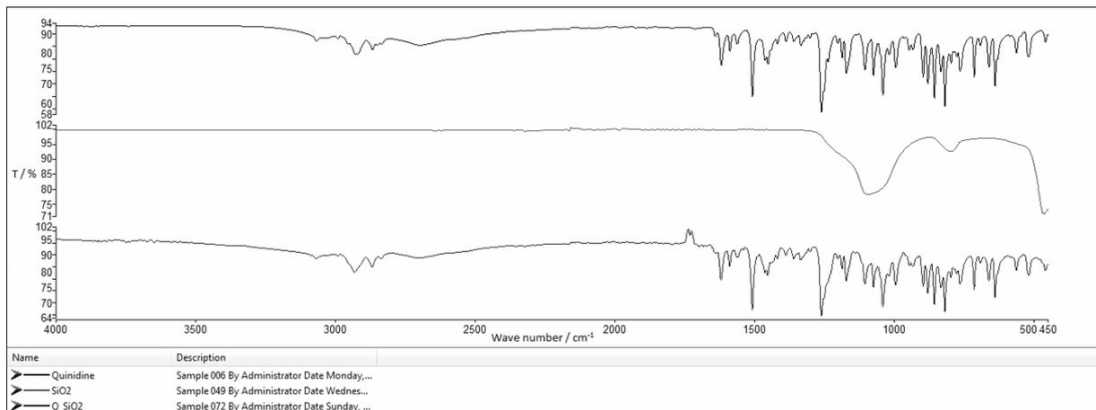
Fig. 2C – FTIR spectra of quinidine, SiO<sub>2</sub> and the binary mixture.
