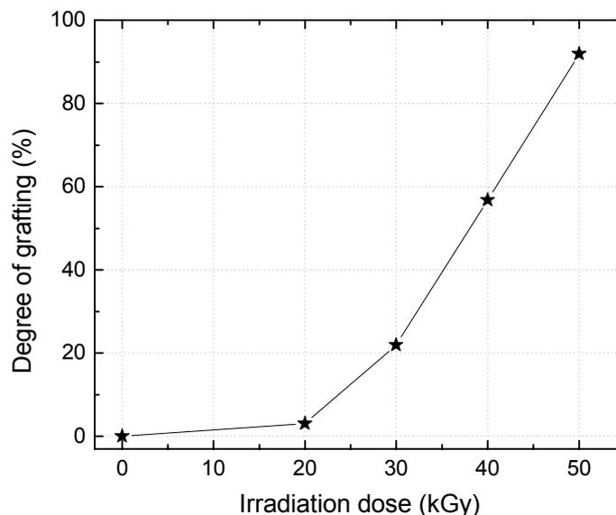
Fig. 6 – Grafting yield onto PE vs. the irradiation dose;  $\text{FeCl}_3 = 1\%$ ; Azole/AAc = 1:3; acetone: water = 30: 70; comonomer concentration = 40%.
