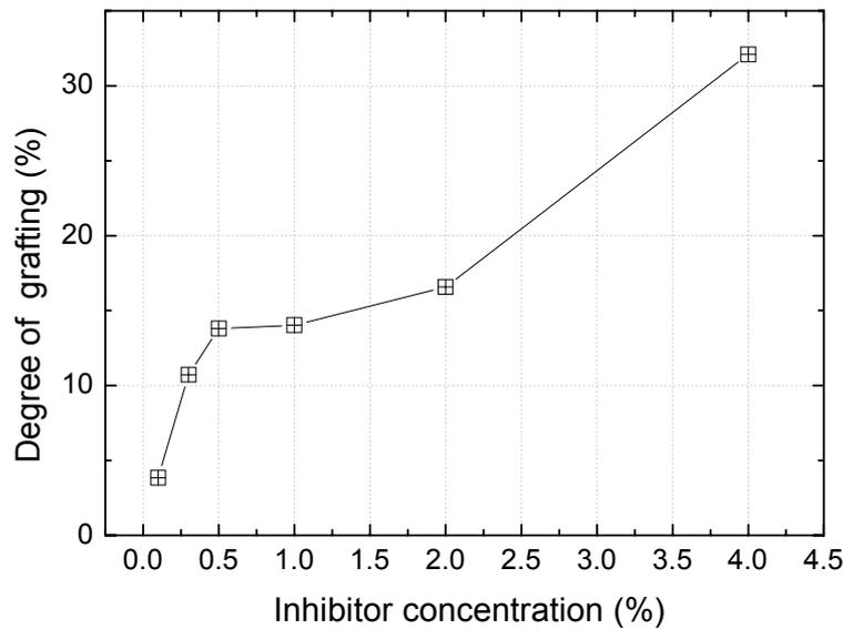
Fig. 2 – Grafting yield onto polyethylene vs. the inhibitor concentration; irradiation dose = 30 kGy; Azole: AAc = 3:1; acetone/water = 30/70; monomer concentration = 20%.
