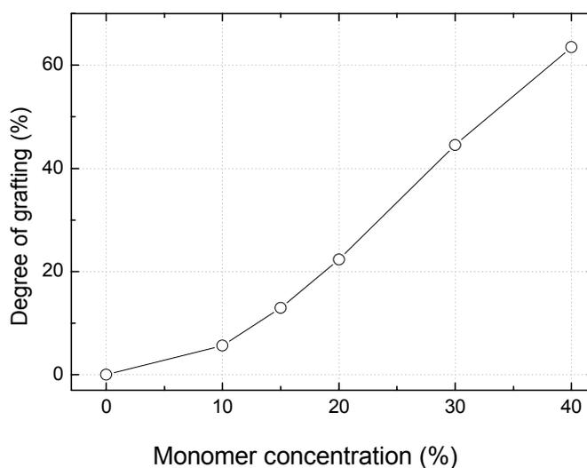
Fig. 5 – Grafting yield onto PE with respect to comonomer concentration;  $\text{FeCl}_3$  = 1%; Azole/AAc = 1:3; acetone: water = 30: 70; irradiation dose = 30 kGy.
