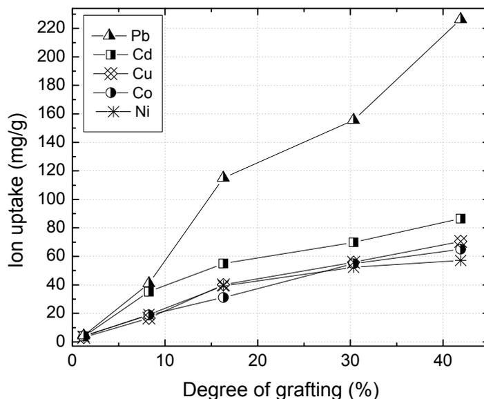
Fig. 8 – Uptake of  $\text{Co}^{2+}$ ,  $\text{Pb}^{2+}$ ,  $\text{Ni}^{2+}$  and  $\text{Cd}^{2+}$  ions versus the grafting yield of PE-g-AAc/Azole; initial feed concentration = 2000 ppm; time = several days; ambient temperature = 22 °C.
