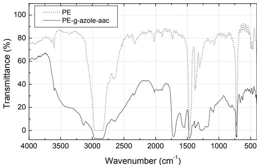
Fig. 7 – FTIR spectra of the original PE and PE-g-AAc/Azole films.
