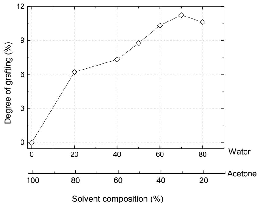
Fig. 3 – Grafting yield onto polyethylene vs. the solvent composition; irradiation dose = 30 kGy; monomer concentration = 20%; inhibitor concentration  $\text{FeCl}_3$  = 1%; Azole/AAc = 1:3.
