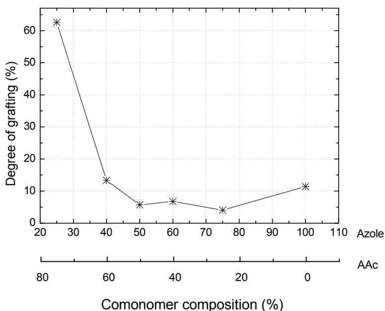
Fig. 4 – Grafting yield onto polyethylene vs. the comonomer composition; reaction parameter: irradiation dose = 30 kGy; monomer concentration = 20%;  $\text{FeCl}_3$  = 4%; acetone/water = 30:70.
