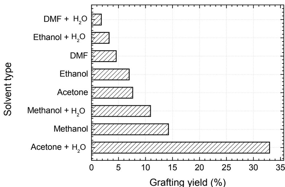
Fig. 1 – Grafting yield for different solvents; the other reaction parameter are constant as follows: irradiation dose = 30 kGy;  $\text{FeCl}_3$  = 1%; Azole/AAc=1:3; monomer concentration = 20%.
