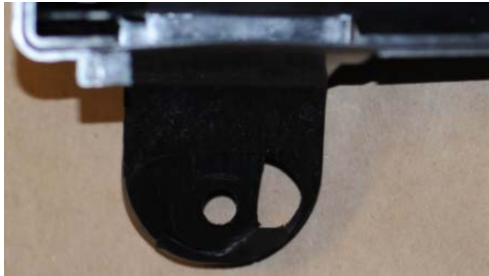
Fig. 1 – Defective part because of crack failure.
