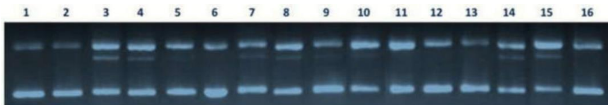
Fig. 6 – “1. \lambda DNA / EcoRI + Hind III Marker; 2. supercoiled DNA control; 3. complex 6 \mu\text{M} ; 4. complex 6 \mu\text{M} + DMSO 0.4 M; 5. complex 6 \mu\text{M} + tert-butyl alcohol 0.4 M; 6. complex 6 \mu\text{M} -sodium formate 0.4 M; 7. complex 6 \mu\text{M} + urea 0.4 M; 8. complex 6 \mu\text{M} + tetramethyl piperidone 0.4 M; 9. complex 6 \mu\text{M} +DABCO 0.4 M; 10. complex 6 \mu\text{M} + TRION 100 mM; 11. complex 6 \mu\text{M} + neocuproine 12 \mu\text{M} ; 12. complex 6 \mu\text{M} + neocuproine 120 \mu\text{M} ; 13. complex 6 \mu\text{M} + neocuproine 240 \mu\text{M} ; 14. complex 6 \mu\text{M} + distamycin 8 \mu\text{M} ; 15. complex 6 \mu\text{M} + methyl green 1.25 \mu\text{g/ mL} ; 16. complex 6 \mu\text{M} + catalase 650 U/ mL”.
