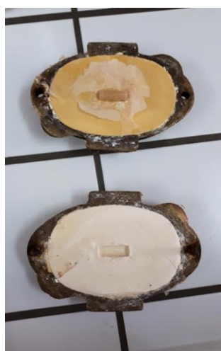
Fig. 1 – Muffle containing a methacrylic resin after polymerization.
