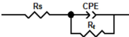
Fig. 7 – Electrical equivalent circuit of the metal/electrolyte interface.
