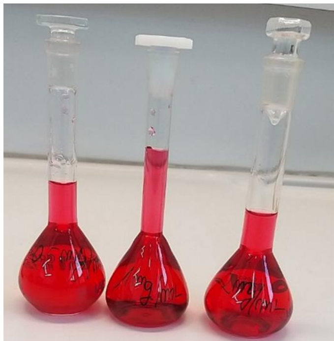
Figure S1. Azorubine-buffered glucose solutions of different concentrations used for intrinsic accuracy testing of the glucometers
